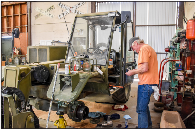
Earl Soladay services the front-end of our forklift.
