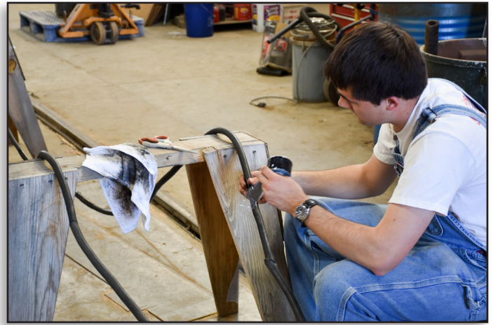
Stephen Hager repairs a locomotive jumper cable.
