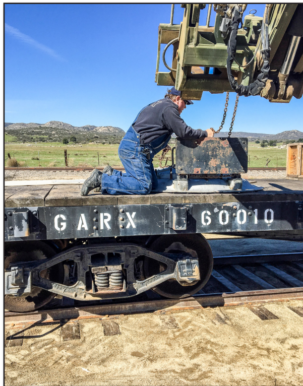
Dave Smith hooking up the smokebox front in preparation for moving it with the forklift.
