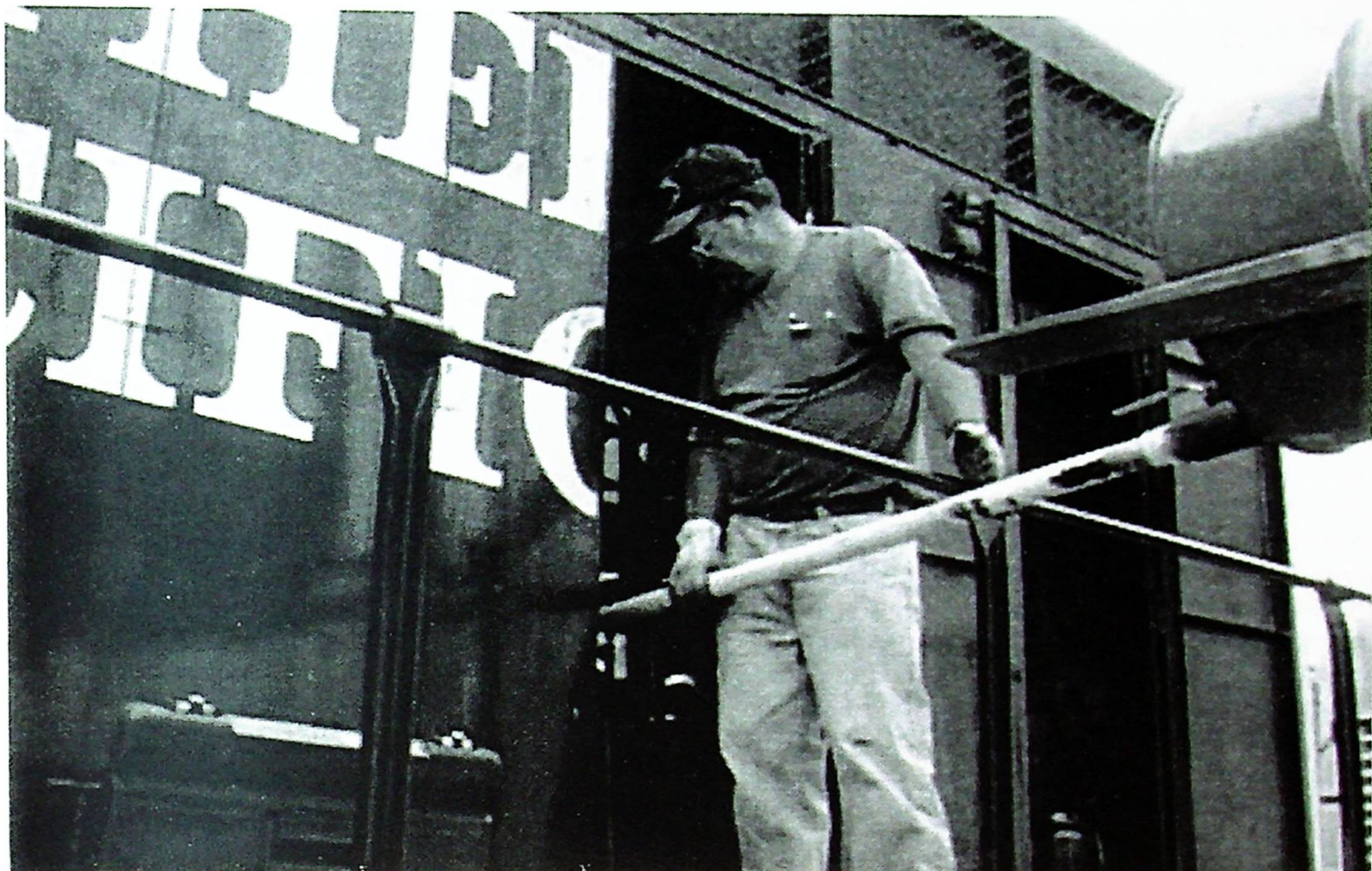
Bill Palmer is shown here in the last stages of an oil change in our GP-9, SP No. 3873. The 55 gallon drum has been hoisted high by the Museum fork lift operated by Ron Hyatt , V.P of Operations . Bill is better known as a steam locomotive expert having served as the Master Mechanic on the restoration of the 300 ton ATSF 4-8-4 No. 3751 for the San Bernardino Railroad Historical Society several years ago. Bill's a machinist of rare talent and we are glad to have him as our Chief Mechanical Officer.
