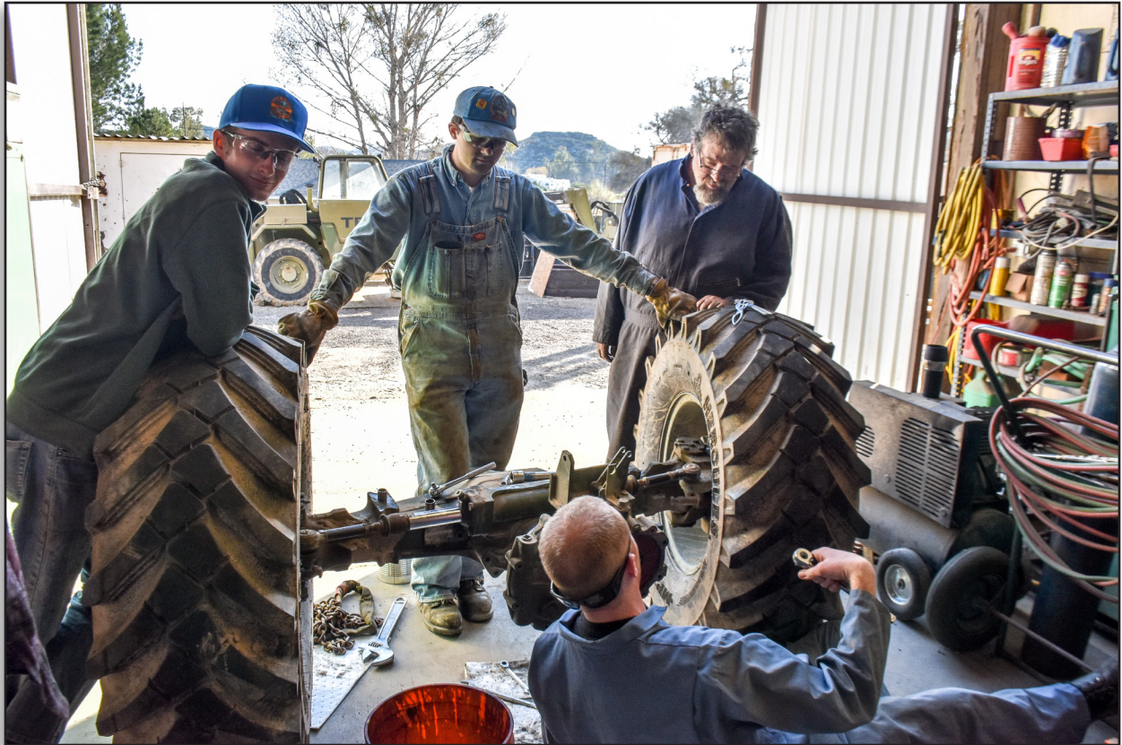
Stephen Hager, Robbie Smith and John Cenkner work on the front axle of the heavy duty forklift while Jarod Black supervises.
