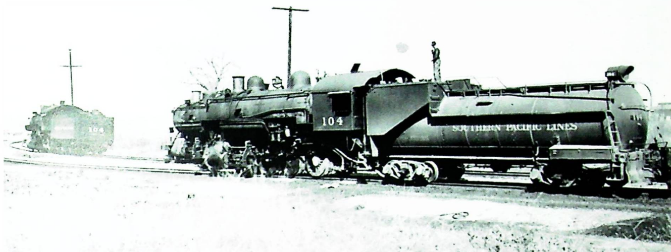
This amazing photo shows the great tender swap actually going down! Both tenders in this picture are numbered 104! In the distance is engine number 2851 now with 104's old square tender. The tender now on 104 is from engine 8381 and has already been lettered for 104. This is a longer version of the Vandy type tender it had when donated to San Diego's railfans in 1955. A third loco can be seen behind 104. This photo was taken by Allen Youell in LA on February 18, 1940.
