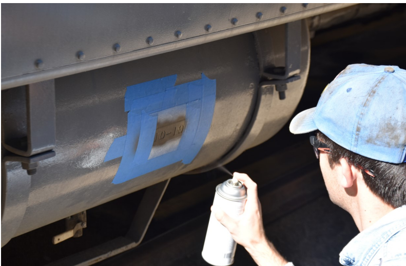
Stephen Hager stencils the COTS date on a railcar signifying that this car has passed its airbrake tests
