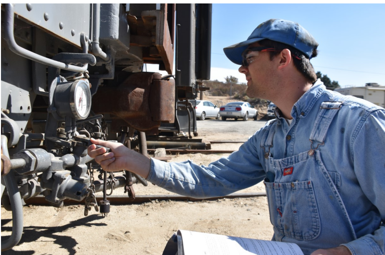
Stephen Hager performs airbrake tests on the railcars used for our North Pole trains
