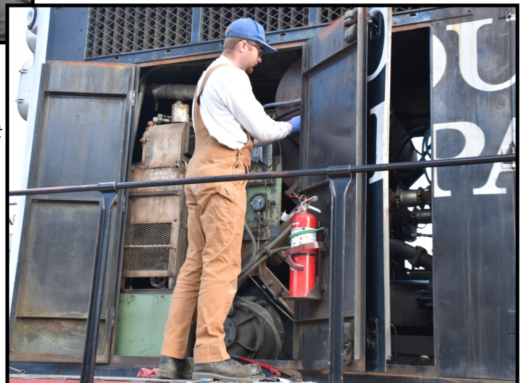
John Cenkner cleans the site glass for the cooling-water tank on SP 3873
