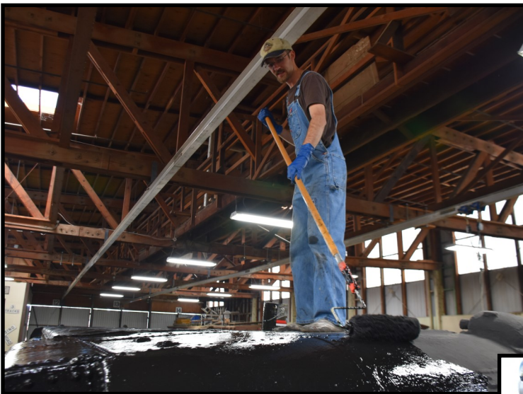
John Cenkner cleans the site glass for the cooling-water tank on SP 3873
