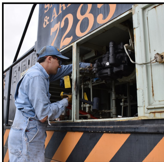
Stephen Hager works on the SD&A 7285 airbrakes
