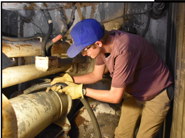
Jarod Black cleaning the inside of the Fairbanks Morse locomotive prior to airbrake work.
