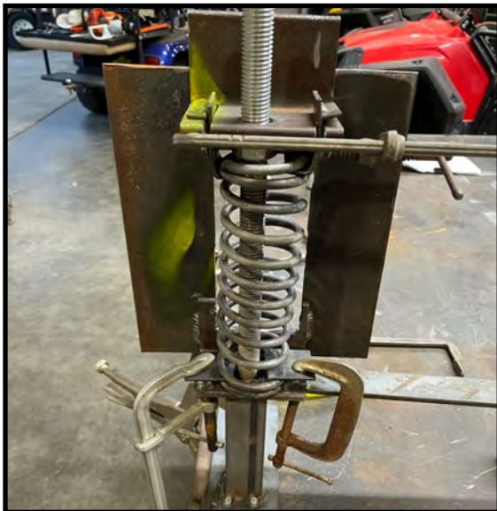
New member volunteer Allen Jones is stretching a donated spring at his home shop in Alpine. The springs will be used for mine train switches
