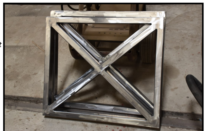
The frames for the battery trays to go into SDA 7285.
