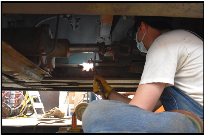
Ron Hyatt cleaning the slack adjuster and prepping it for overhaul.
