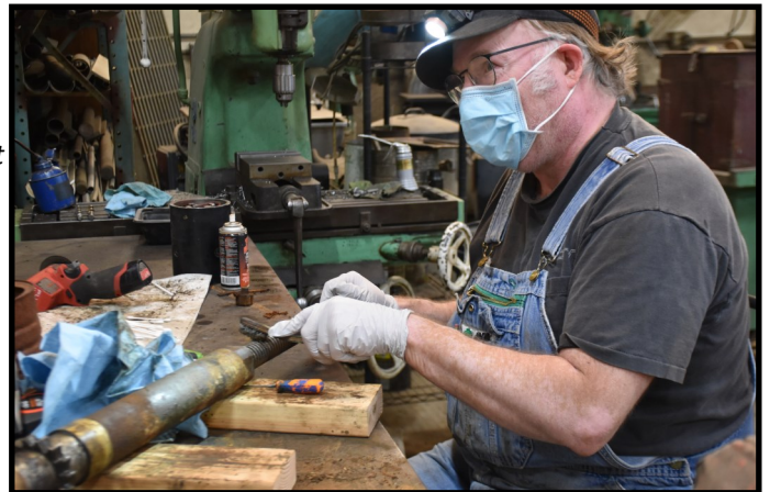
The rebuilt slack adjuster ready for reinstallation.
