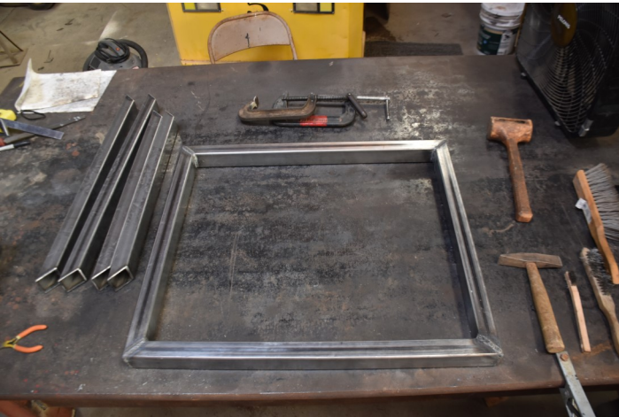
Initial framing for battery trays
