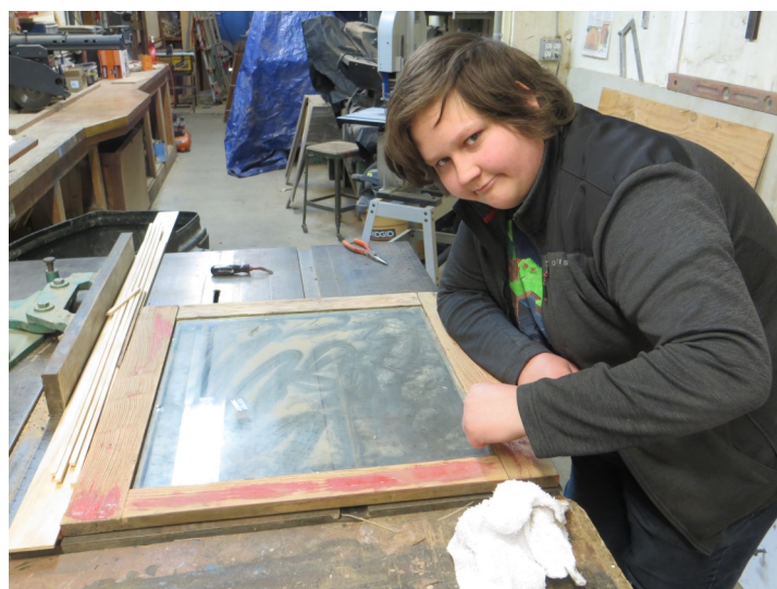
Ian Hyatt is working on the window frames for the C&O caboose inside the wood shop.
