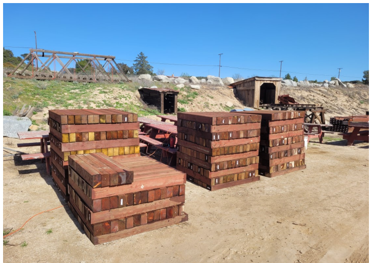
Jim Lundquist is cutting 16 foot timbers into 4 foot ties. Photo by Steven Pohjola 4/7/22
