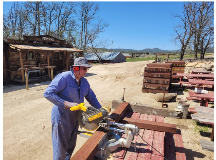
Jim Lundquist is cutting 16 foot timbers into 4 foot ties. Photo by Steven Pohjola 4/7/22
