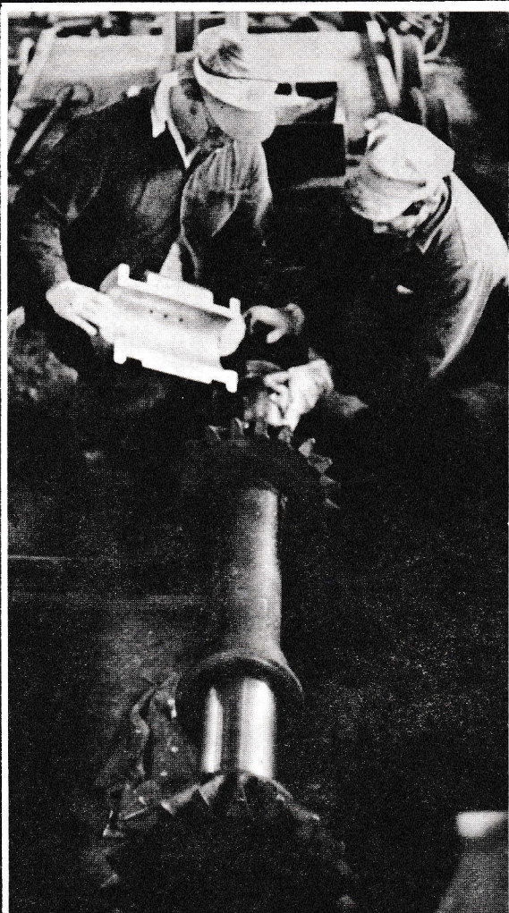
Ken Helm and John Ashman are shown here servicing the bearing brass for our Shay's three drive shafts that are being carefully cleaned and repacked.
