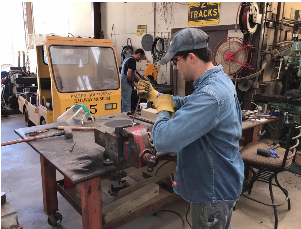
Stephen Hager fabricates a handle for a die while Martin Caestecker cuts steel on the chop saw. Photo by Frank Najera.
