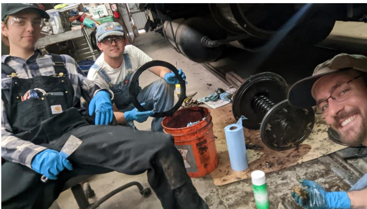
Left - Volunteers Paul Bandemer, Stephen Hager and Martin Caestecker are working in the shop performing servicing one of SD&A 253's brake cylinders.
