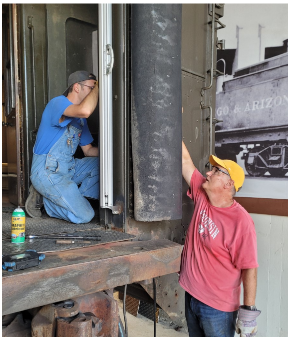
(left) Martin Caestecker and Richard Ulrich install a new hand brake on a SD&A coach inside the Shop Building.
