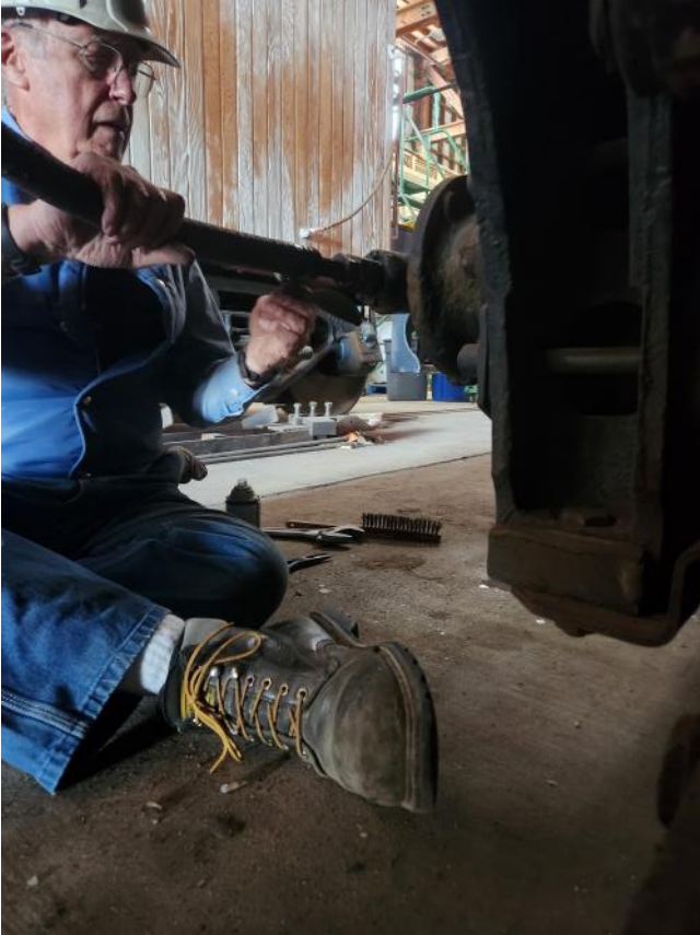
Rich Paulus installing the speed indicator cable
