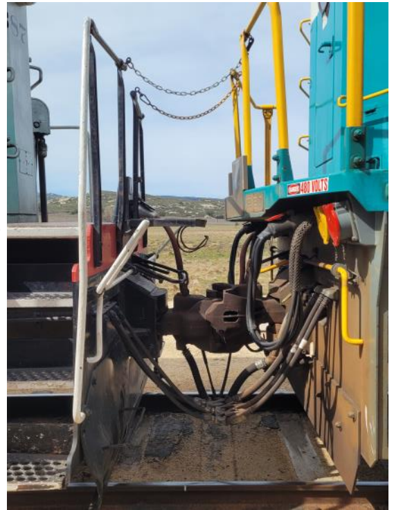
Electrical and air hose connection ("MU" - multiple unit) between Coaster 2103 and SP 3873 allowed 2103 to control 3873, which powered the train
