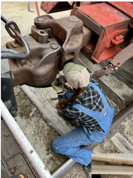
Left - lacing up the air hoses.
