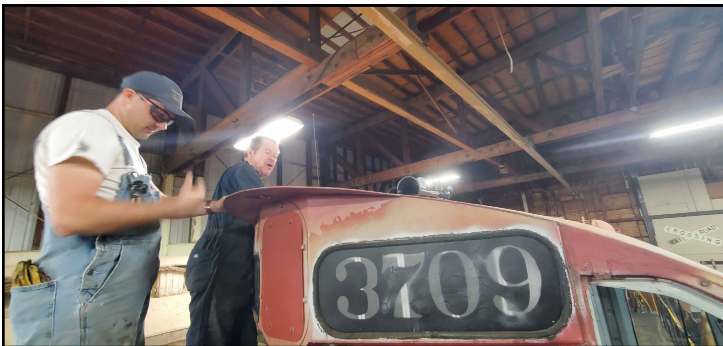
Stephen Hager, Jaden Soroka and Geoff Patrick are investigating areas of corroded steel to cut out and replace on the cab of the SP #3709.
