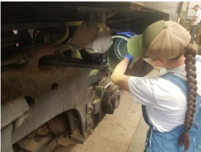
Grace Brown working on brake cylinders on SP 3709 Photo by Stephen Hager
