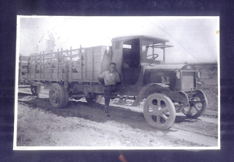
Old GMC Truck with a load of cotton bales. Note the hard Rubber tires, the hand crank on the front to start the Motor, and the windshield that opens for fresh air.
