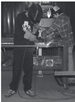
A section of the framework for the stage gets welded together.
