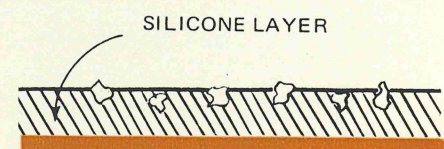
FIGURE 5 GLAZE SURFACE By applying a Silicone grease coating to a new insulator it acts as a parting agent in keeping dust particles out of contact with the fresh glazed surface.
