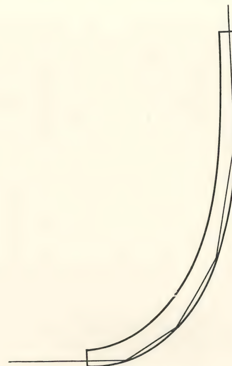
FIG. 15. Total internal reflection around a bend in a quartz tube.
