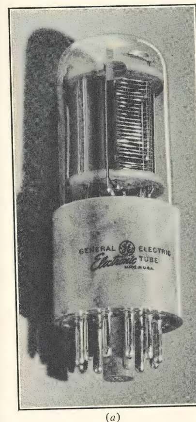
FIG. 4. Photomultiplier tube. a. Photograph. (Courtesy of General Electric Co.) b. Schematic diagram.
