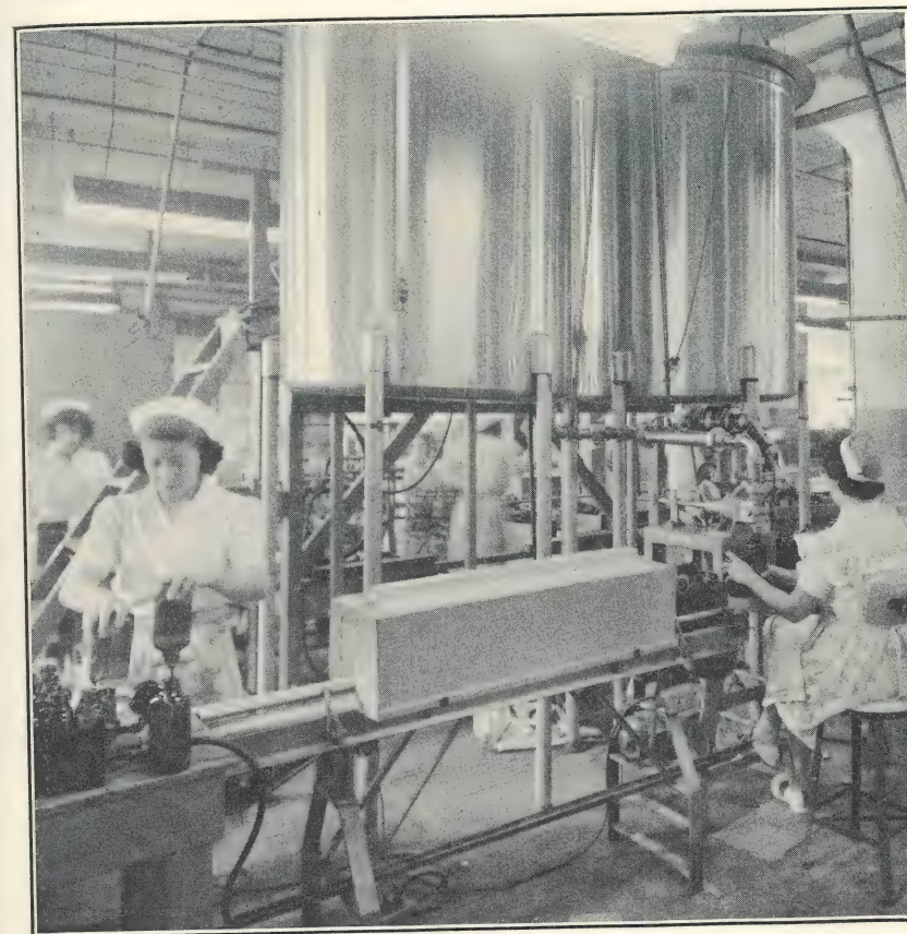
FIG. 7. Bottles on conveyer pass through tunnel under high intensity ultraviolet radiation before filling. (Courtesy of General Electric Co.)
