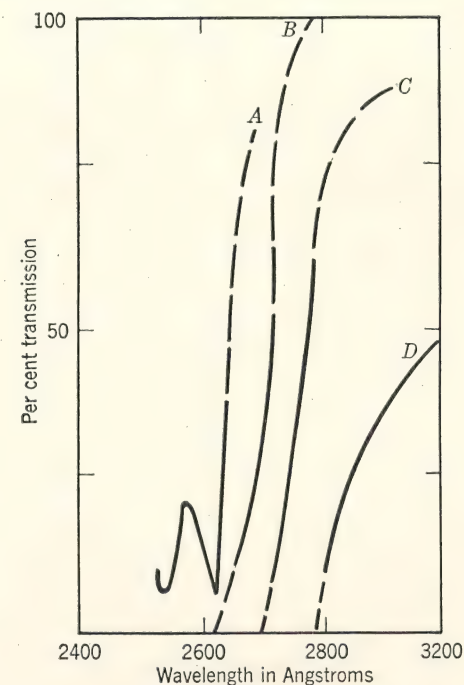
FIG. 12. Transmission of filters of various concentrations of benzene dissolved in octane. A. 1.0 grams per liter. B. 9.1 grams per liter. C. 100 grams per liter. D. Undiluted. (A. N. Bass, J. Optical Soc. Am. , 38 , 977, 1948.)
