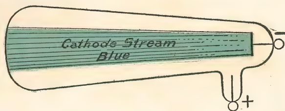
FIG. 29.—Illustrates the original Crookes tube, the X-ray being generated at the end of the tube where the cathode stream strikes the glass. It was from a tube of this type that the X-rays were first obtained. Owing to the many sources of the rays, the pictures were very indistinct.
