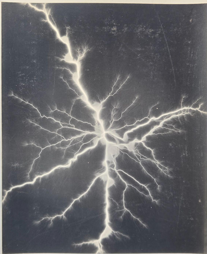
No. 25. STRUTED SPIRAL DISCHARGE. Not Enlarged. A discharge from a metallic point upon a horizontally suspended photographic plate. Transformer from 3. American, 110° volts.
