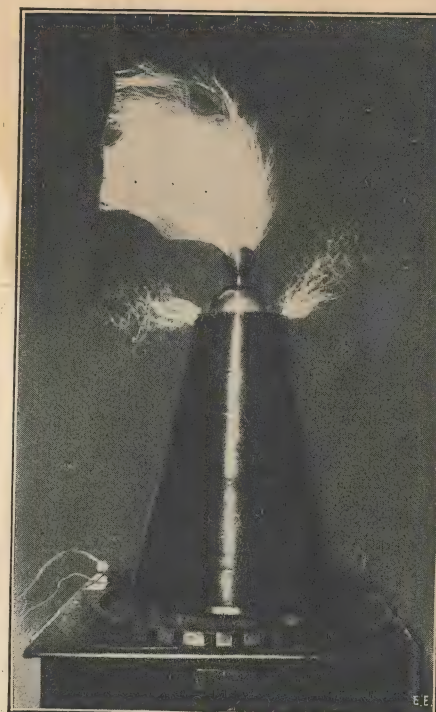
Fig. 2. Another View of the Strong High Frequency Coil Producing a Perfect Sheet of Flaming Sparks to a Grounded Conductor. The Exciting Energy is but 1 Kilowatt.
