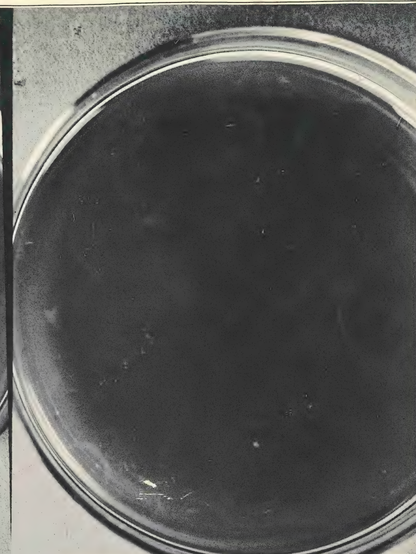
6-A B.coli Through Pharyngeal Applicator - Quartz tipped Distance - grid to culture 6-1/8 inches Time - 3 minutes
