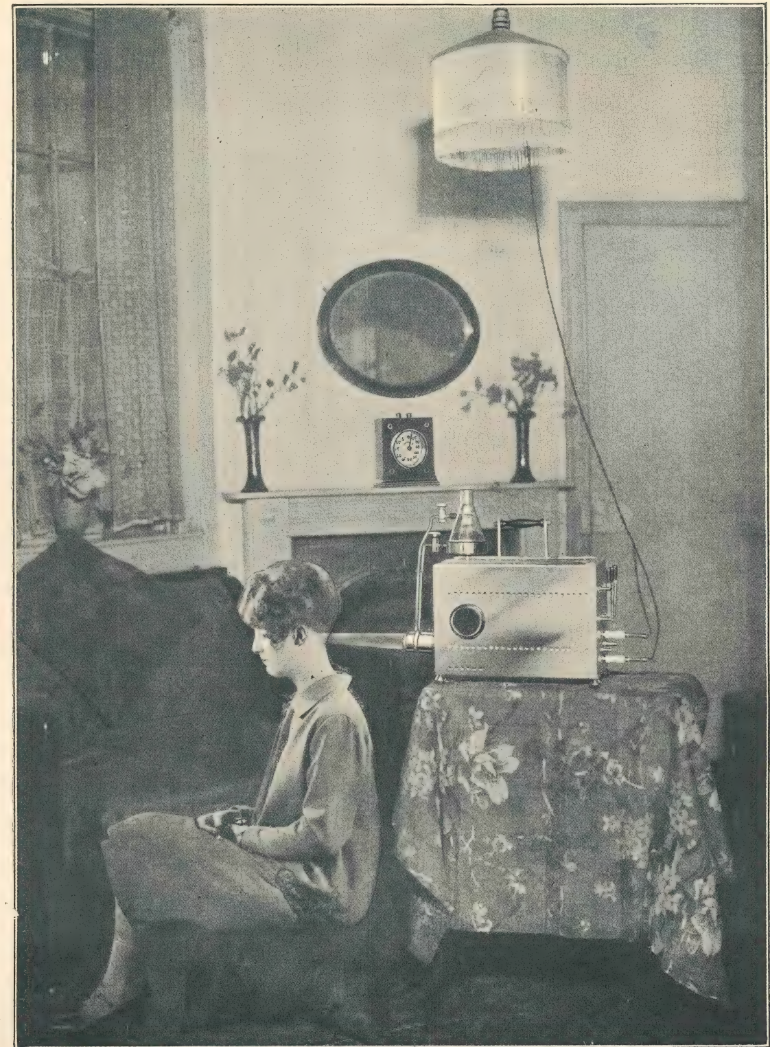
The illustration shows the water-cooled quartz concentrator in use in conjunction with the "Ajax" Portable Arc Lamp. A continuous circulation of water on the thermo-syphon principle keeps the rays perfectly cool. It will be noticed that in this instance the lamp is being used from the ordinary house lighting circuit.
