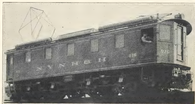
Figure 18—110-Ton Baldwin-Westhouse 11,000-Volt, Single-Phase 25-Cycle Locomotive, Equipped with Four Westinghouse 340-h. p. Single-Phase Motor Units and Unit Switch Control
