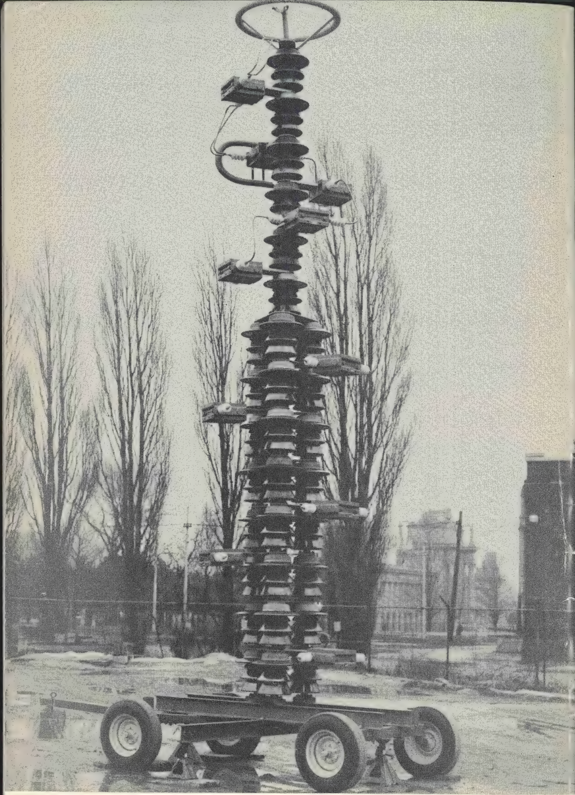
Coupling capacitor for radio-noise measurements at the Coldwater ehv test project, in assembly stage. Designed for operation up to 350 kv to ground, the capacitor will be movable for convenience of measurement on each phase.
