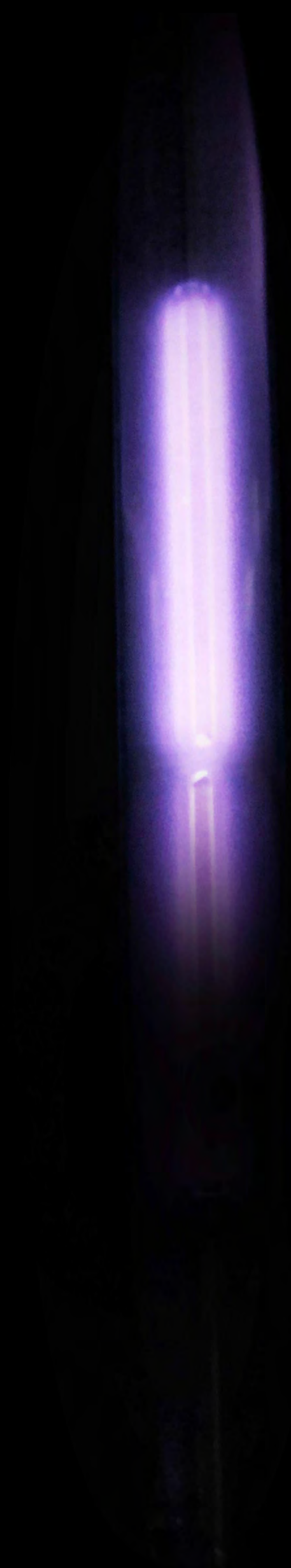
Ruhmer's Ondoscope: If the source isn't a pure direct current (inverse discharges are present) a portion of the other electrode will light as well. On alternating sources both poles light equally.
