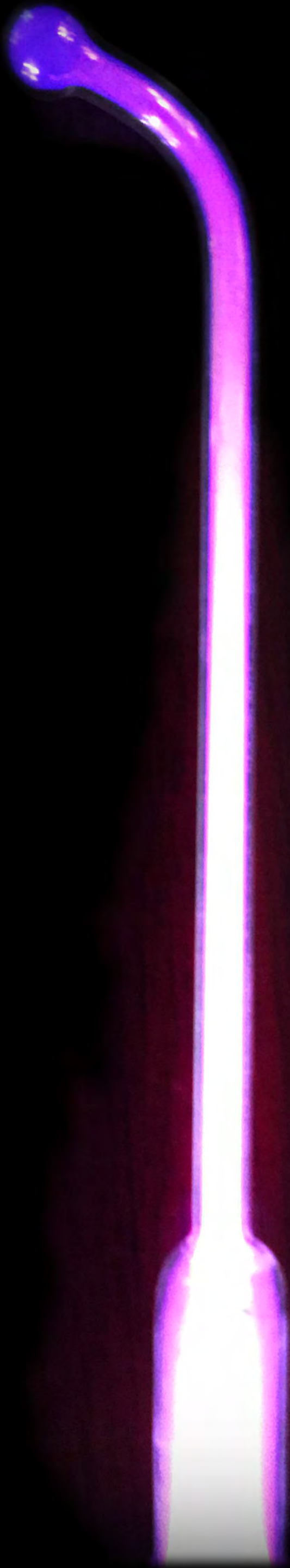
Diathermy Glass Vacuum Electrode: Geissler tube used for treatment of the throat
