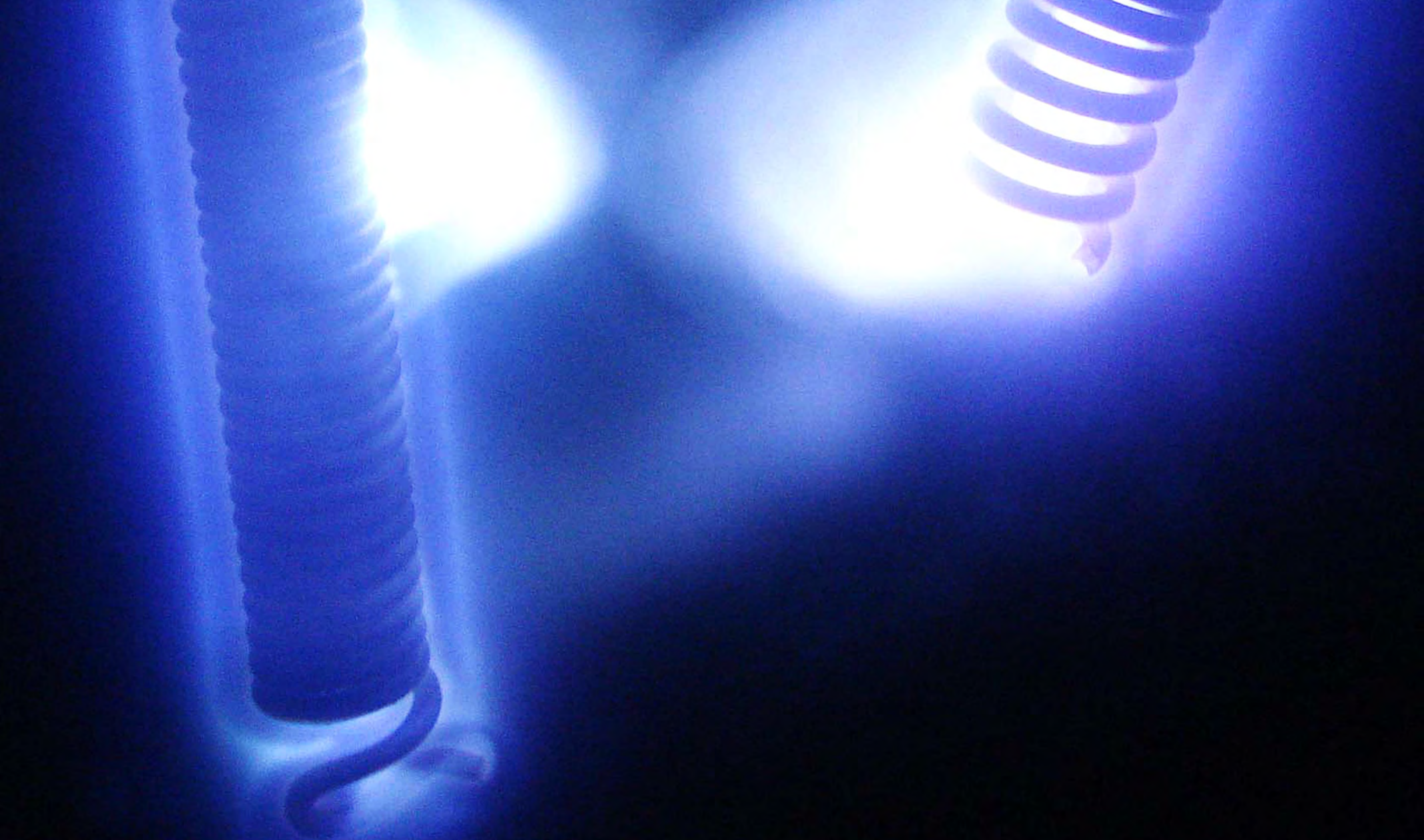
Electricity in a bell jar: Light in a partial vacuum, 1/100,000th of an atmosphere
