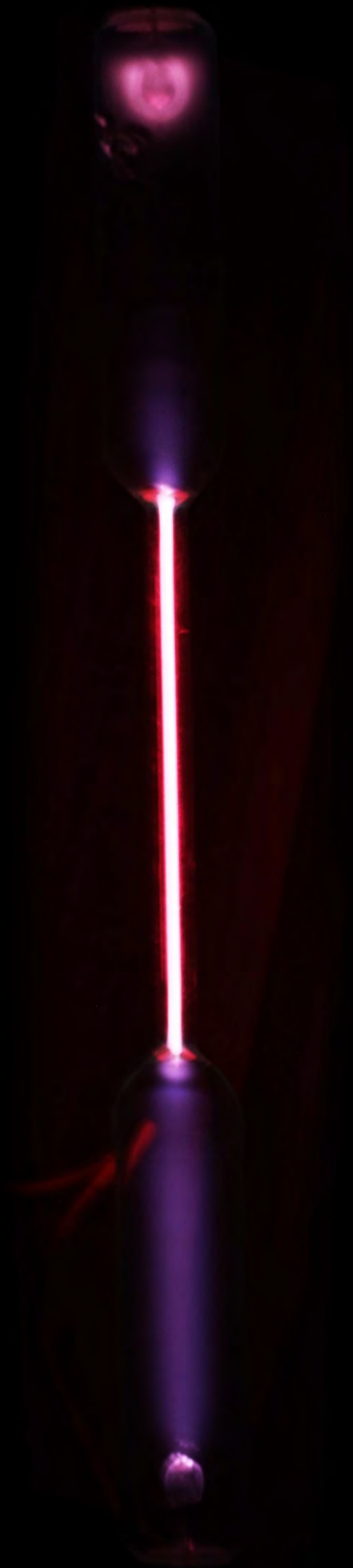
Spectrum Tube: Geissler Tube used to study wavelengths of light emitted by certain gases. This tube contains nitrogen gas.
