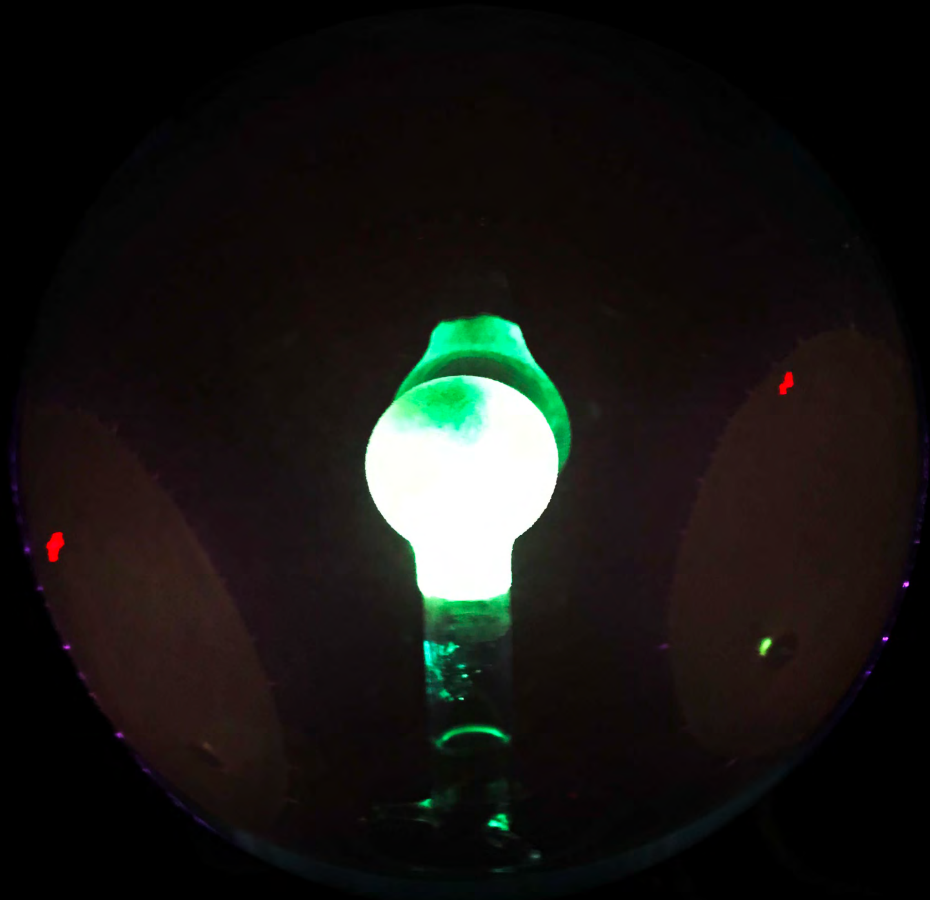
Ebert Lamp: Phosphorescent Lamp using external electrodes powered with high frequency currents
