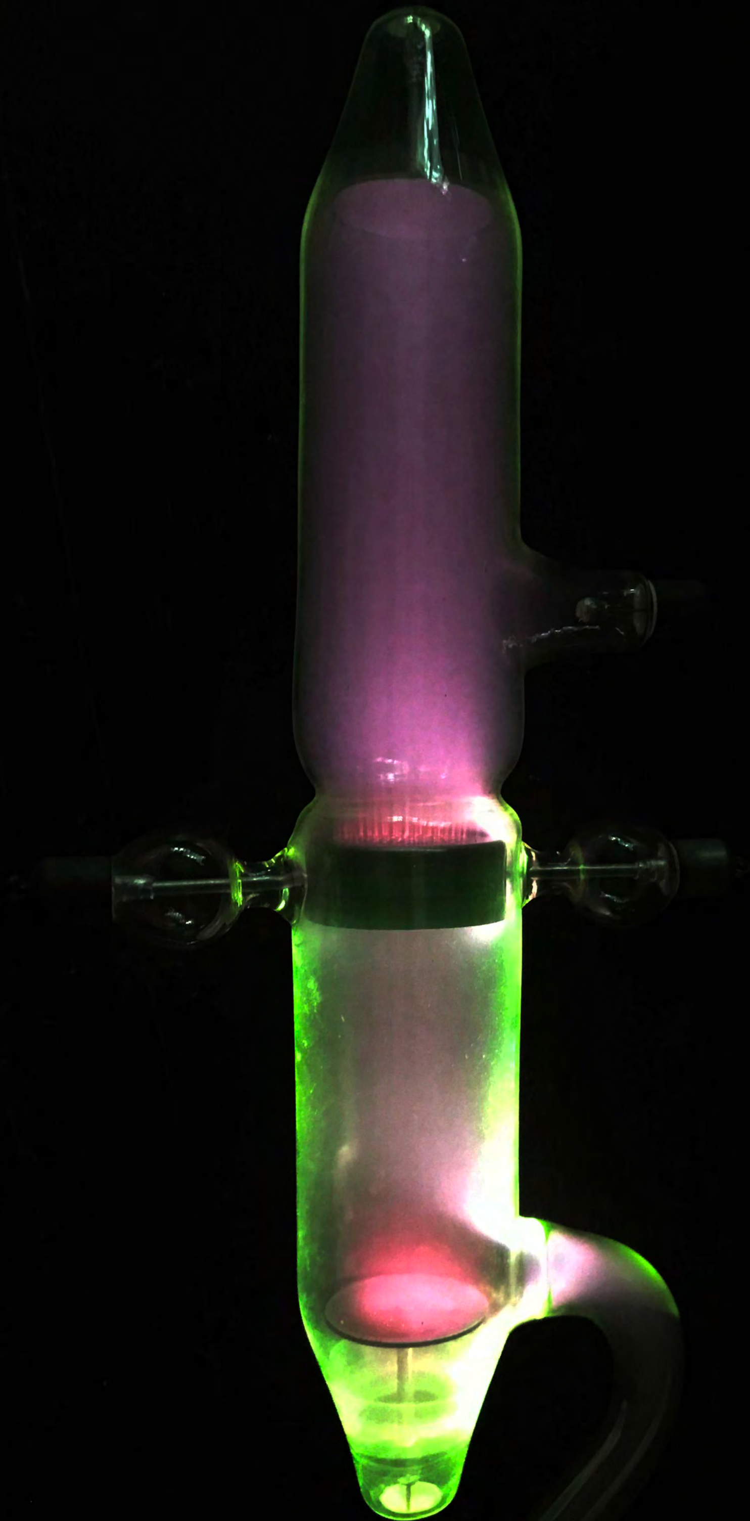
Anode Rays accelerate positive ions in the tube combining them in clusters that become attracted to the cathode.
