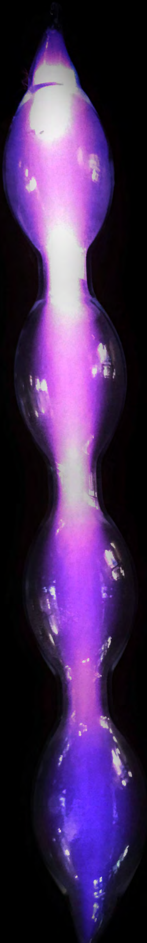
Electrodeless Geissler Tube made by Jeff Behary to demonstrate Tesla system of lighting. Residual air in a partial vacuum positioned in the nearby electrical field of a Tesla Coil.
