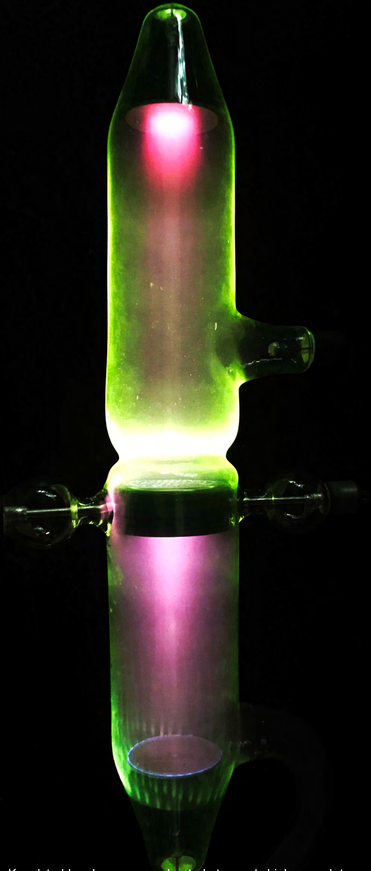
Canal Rays or Kanalstrahlen: Ions are accelerated at speeds high enough to cause fluorescence in the tube as the different molecules change energy states.
