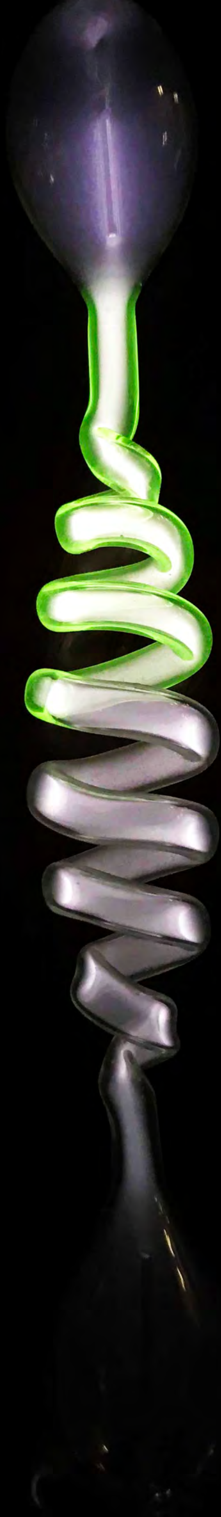
Geissler Tube: Early electric lamp using residual air in a vacuum. Made with uranium oxide glass fused to soda lime glass.
