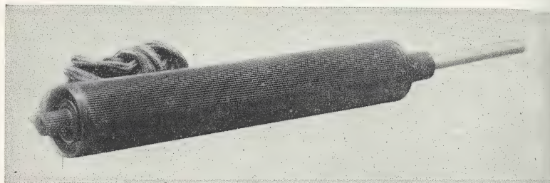
FIG. 71.—A high tension spark coil for testing the vacuum system. The knob at the end is used to control the intensity of the spark, which appears at the metal tip of the device.
