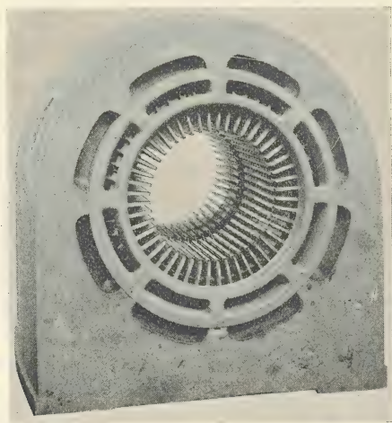
FIG. 30—SAME MACHINE AS SHOWN IN FIG. 29 BEFORE WINDING
