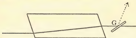
Fig. 88. The figure shows a polarised ray meeting a piece of plane glass, and experiencing a feeble reflection: nearly all the light goes through. But if the piece of glass - or the Nicol - is turned through 90^\circ about the line of the ray which is passing through it in the diagram, the reflection becomes strong. The experiment of Malus.
