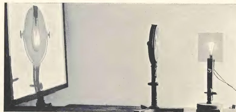
B. This photograph shows on the left the inverted image of a filament lamp which stands upon the right; the image is produced by the lens in between. The square screen in front of the filament lamp was put there during part of the time while the photograph was being taken in order to cut down the light from the filament, which otherwise would have been too strong for the photographic plate. The inverted image of the filament on the screen is due to the original filament itself; but the inverted shadow of the lamp bulb is due to a light which was placed on the right, out of the field of the photograph. The same external light casts a shadow of the lens and stand which are right way up, because the rays have not been through the lens. (p. 45)
