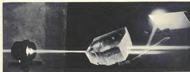
B. The block of Iceland Spar breaks up the original light ray into two. The line joining the two spots where they emerge is parallel to the line bisecting the obtuse angle of the face on which the spots lie. The light vibrations in the lower ray, which is the ordinary ray, are perpendicular to this line, that is to say, they are parallel to the piece of reflecting glass. A portion of the ray is reflected as the figure shows. The vibrations in the upper ray, which is clearly the extraordinary ray because it is out of alignment with the original ray, are parallel to the line joining the spots. It is not reflected. (p. 178)
