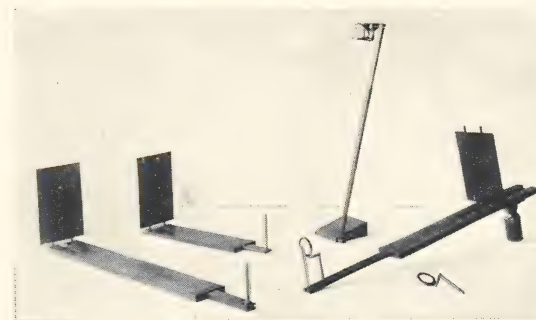
C. Eriometers made and used by Young. In each of these is a fibre holder, a screen with small holes and a sliding scale. The mode of use is described on p. 162.
