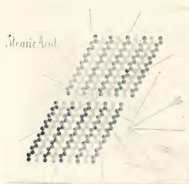
B. The arrangement of the molecules in a crystal of stearic acid. Each zig-zag represents the carbon atoms of a single molecule. The distance between the centres of two neighbouring carbon atoms is 1.54 Angstrom Units, as in diamond. The two models A and B are built on different scales. The terminal groups and the hydrogens are not shown. (From a diagram due to A. Muller, Davy Faraday Laboratory). (p. 249)
