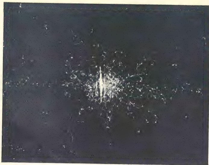
A. In this photograph a fine pencil of rays proceeding from right to left meets a copper screen. It excites a cloud of electrons in the copper; and it will be observed that it has a tendency to carry the electrons with it. There are more on the side where the X-rays emerge after passing through the screen than on the side where they enter. (p. 272)
