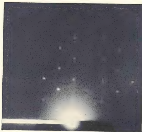
B. A photograph due to the diffraction of electrons (G. P. Thomson.) A stream of electrons has been made to fall upon the surface of a crystal, and the photograph has been placed so as to receive the diffracted beams. (p. 276)
