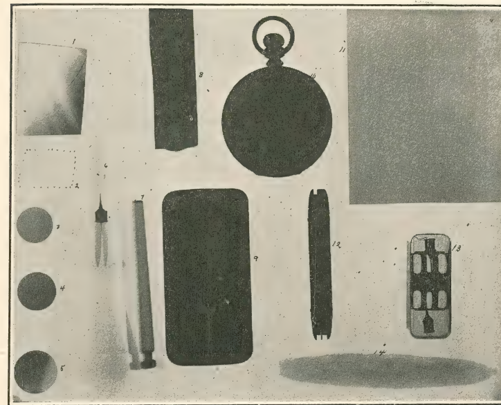
Fig. 2.—From a Skiagraph Made by Dr. A. C. Geyser, Showing Varying Transmissions of the X-Ray of Different Substances.
