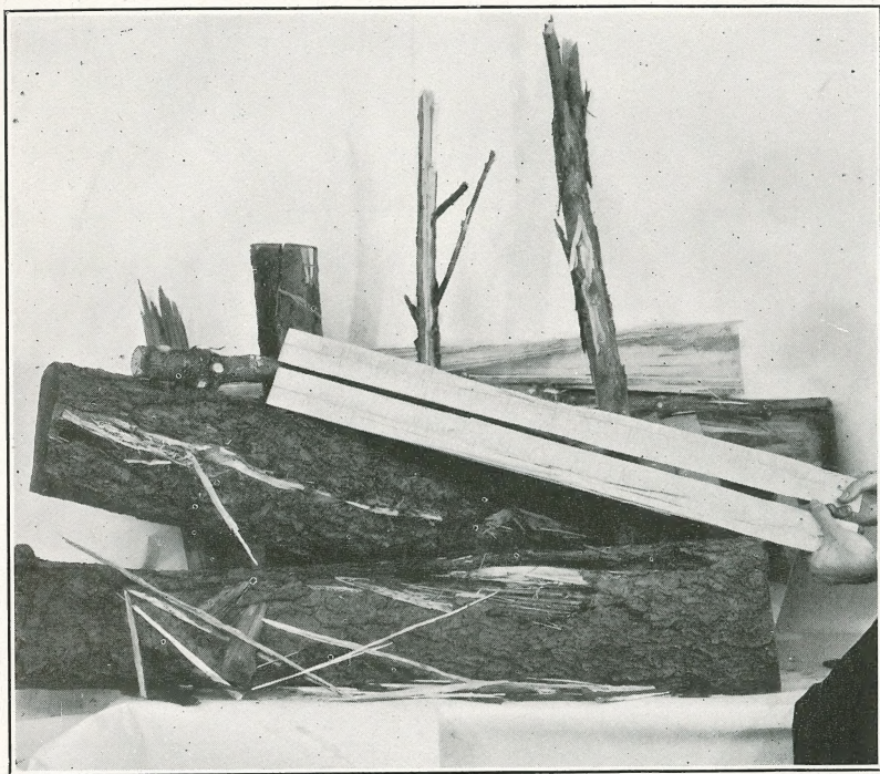
FIG. 8.—WOOD SPLIT BY ARTIFICIAL LIGHTNING
