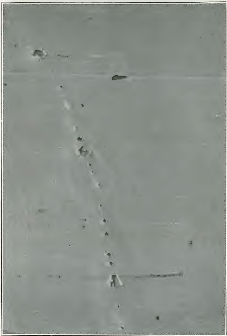
FIG. 9.—METAL "PUNCTURED" BY LIGHTNING
