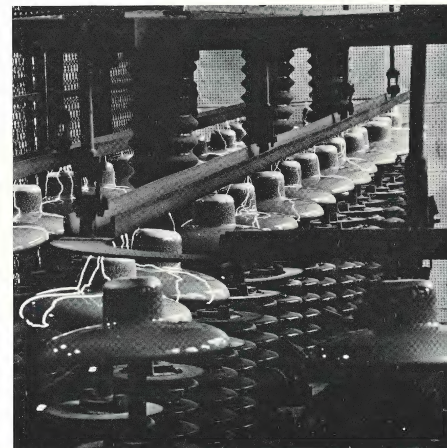
Portion of the endless conveyor that gives every O-B suspension insulator disc a five-minute exposure to full flashover voltage. Five seconds of this test is at 200,000 cycles; the remainder at 60 cycles. This eliminates any defective pieces before they go to assembly. Note that the absence of the cap in this test extends the striking distance over the porcelain, and increases flashover voltage beyond that which is normal for the assembled insulator.
