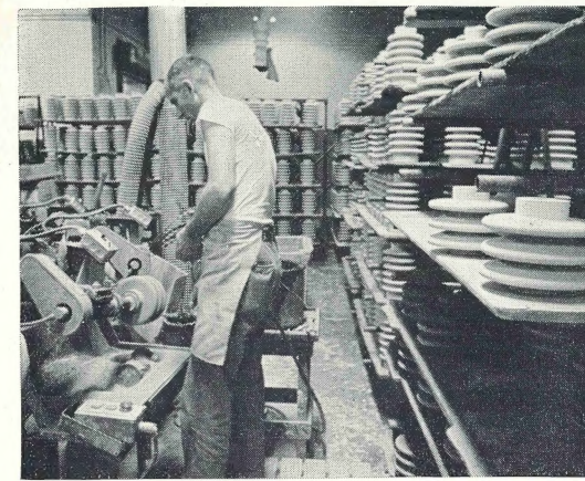
Operator of semiautomatic finishing wheel loads post shapes on machine, inspects them, and performs finishing, glazing, and sanding steps.
