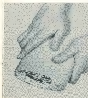
Using the extended foil principle already proved successful by ASEA (Swedish General Electric), Varex element has a uniform mat of aluminum at each end for making electrical contact with metal plate. This type of contact minimizes current density in the element since the greatest distance current must flow is about the width of the aluminum foil.
