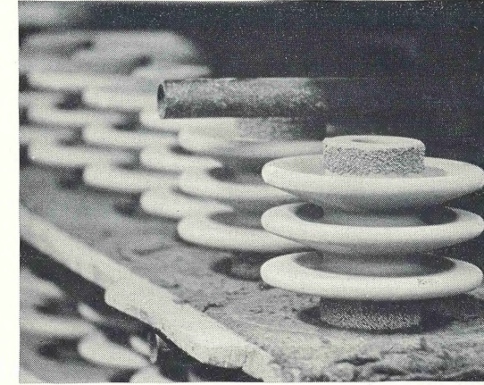
These clamptop distribution line post shapes are finished and ready for kiln firing.
