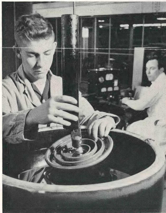
Comparison of results from the oil puncture test with historical values is one measure of quality and expected service performance.
