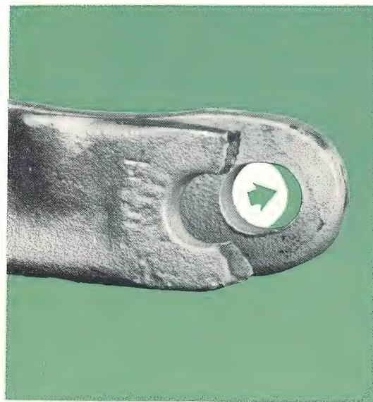
Under tremendous stress, malleable iron strain clamp takes considerable deformation and stretching prior to failure. Note the extent of elongation in the rivet hole before fracture.
