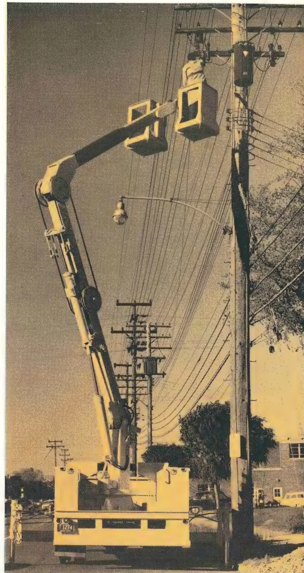
Holan Elbow -- the first aerial elbow with aircraft-type cable controls -- brings new ease of operation, low maintenance and safety to high-up work. Half of upper arm (and sections of the cable controls) are made of fiber-glass-reinforced plastic to provide extra insulation for protection -- the first unit in the industry to offer this as standard equipment.
