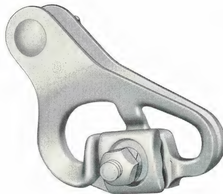
Number 80500 - weighs 1.3 pounds and effectively holds conductors with diameters ranging from .12 inches to .38 inches; ultimate strength of the clamp is 8000 pounds.
