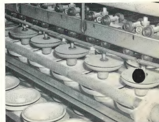
After passage through the mold release dryer, insulator shapes are gently removed from the molds by vacuum lift devices and then conveyed through the final drying cycle. Vacuum lifts are completely automatic, far more delicate and precise than any human hands.
