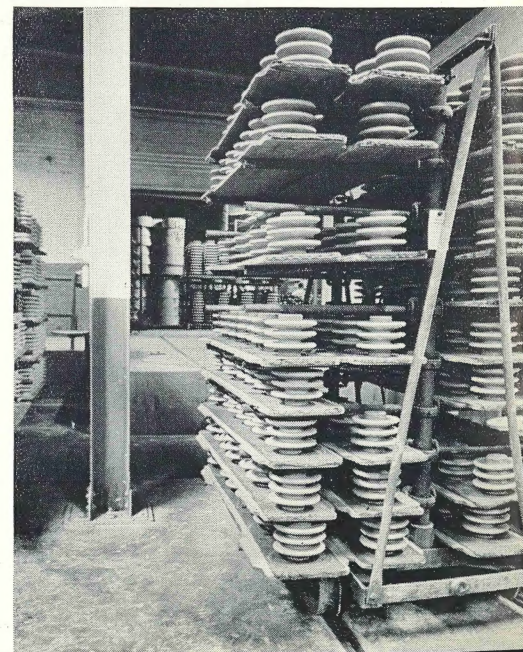
Kiln car loaded with tietop distribution line post bodies waits in line to begin vitrification firing in tunnel kiln.
