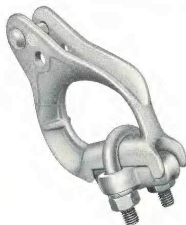
Number 78500 - offers a reversible clamping piece with a U-bolt fastening assembly. Clamps weigh 3.9 pounds and are rated at 14,000 pounds ultimate strength. Conductor diameters range from .16 inches to .55 inches.
