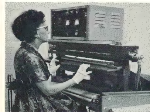
Insulation strength of each element is verified before pack is assembled.
