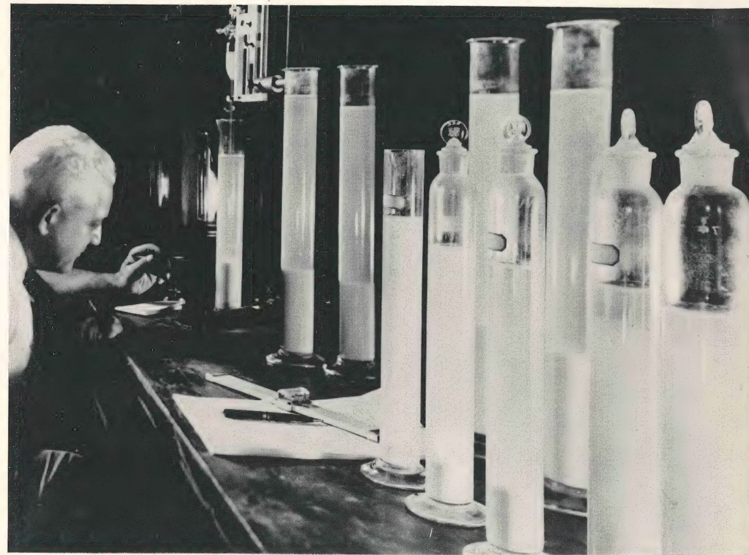
Grains of clay, feldspar and flint are the "building blocks" with which porcelain insulators are made. Grain size affects homogeneity; homogeneity affects mechanical and electrical characteristics; so we start by checking the grain size of our ingredients.
