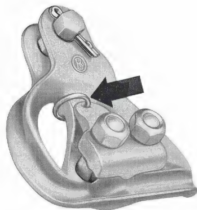
Special, stainless steel spring; see arrow.
