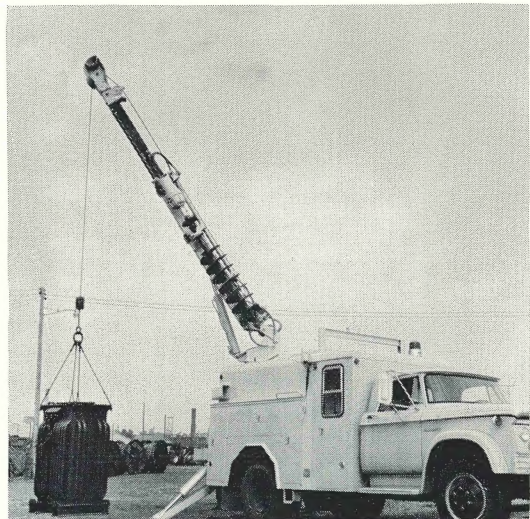
SOLUTION: Override the overload device, retract boom, lower.
