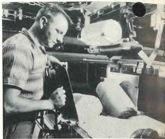
Clay banks arrive on overhead conveyor from clay department and are automatically fed into this vacuum pug mill. Mill removes all air from the clay prior to shaping.
