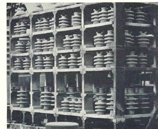
Kiln car loaded with tietop distribution line post bodies waits in line to begin vitrification firing in tunnel kiln.
