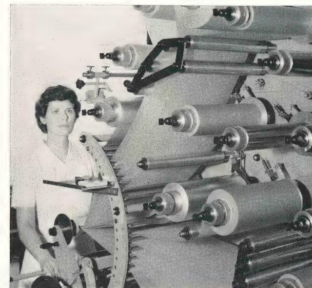
Winding of Varex elements can be done continuously under the same tension since there is no need to interrupt the winding operation to insert contacts. Operator's hands never touch the active dielectric in a Varex element.
