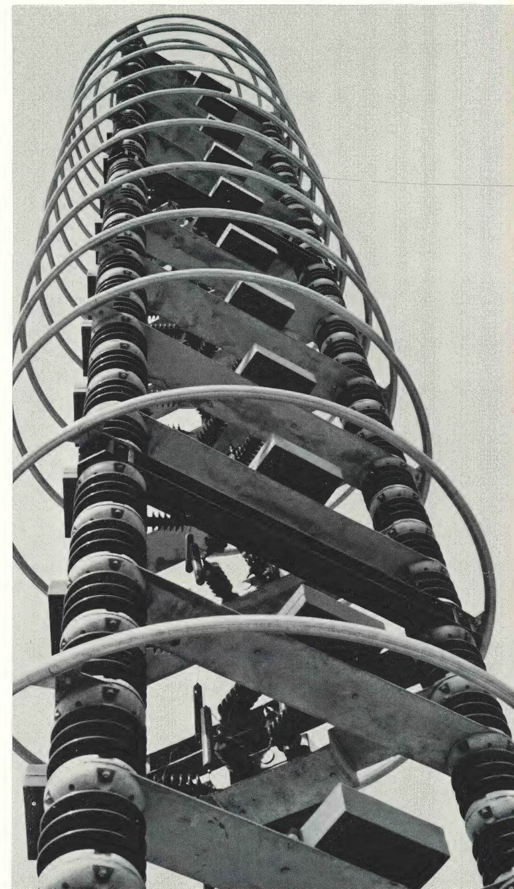
Figure 4 - Fifty-foot loading capacitor and voltage divider tower accommodates helical series circuit of 40 high-voltage capacitors used for switching surge testing up to 3200 kv.
