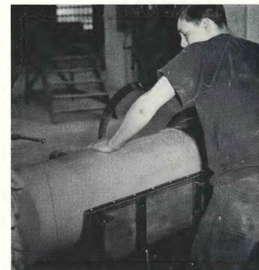
Clay blanks are extruded for future trimming into line posts.
