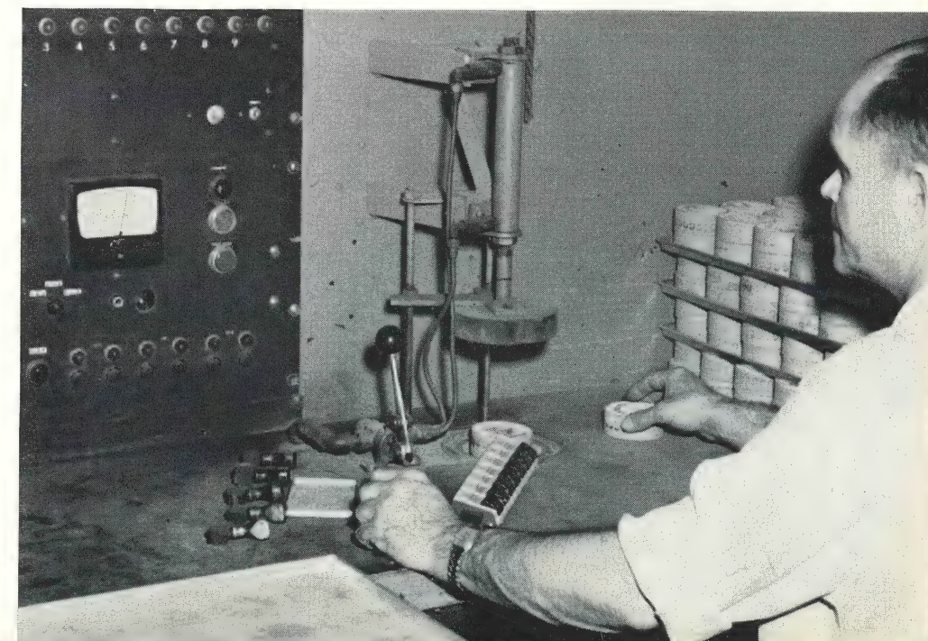
FIGURE 3 Valve blocks for GP intermediate arresters are formed and fired from special compounds, then electronically tested and given pre-conditioning surges for the purpose of improving durability characteristics.
