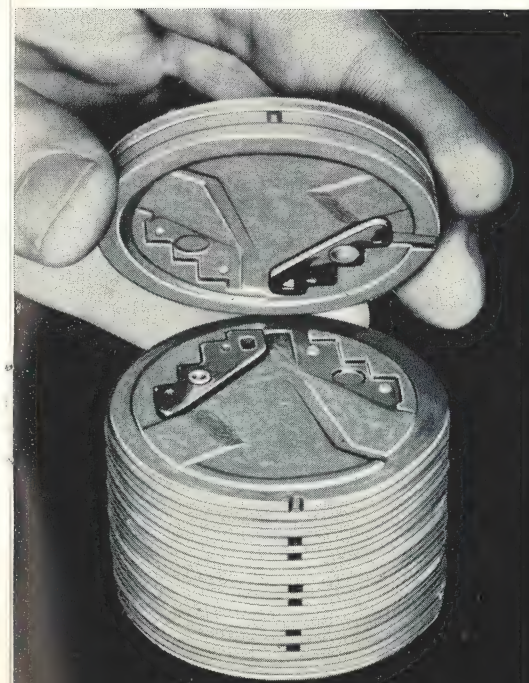
FIGURE 2 The current-limiting Dynagap element consists of a compact stack of thin discs which position the gap electrodes and provide the arc-cooling cavities during interrupting cycle.
