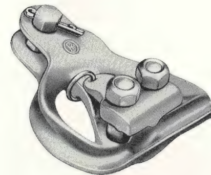
Universal Clamp Number 88500 holds conductor diameters of .20 inch to .50 inch. It has an ultimate strength of 10,000 pounds.
