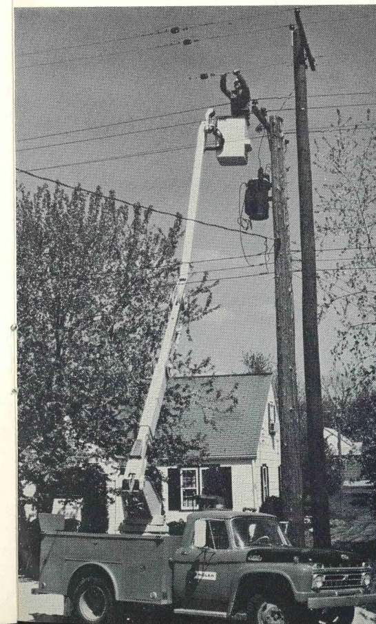
Mounted on either a 60- or 84-inch CA chassis, the Bronco 89-36 includes an integral torsion-bar stabilizer system for assured stability without outrigger jacks — keeps set-up time to a minimum. The optional fiberglass lower-arm insert isolates ground personnel and "sidewalk superintendents" electrically.
