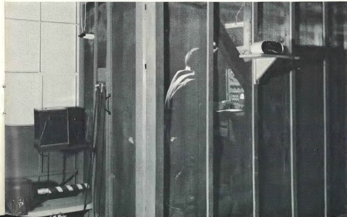
Great flexibility of the 3,000-kv research impulse generator often calls for unusually fine technique in the production of pure test data. This elaborately shielded room can operate without the entrance of a single wire, except for the triple-shielded test lead. Instrument synchronizing signals travel on light beams, and service power can be generated within the room.
