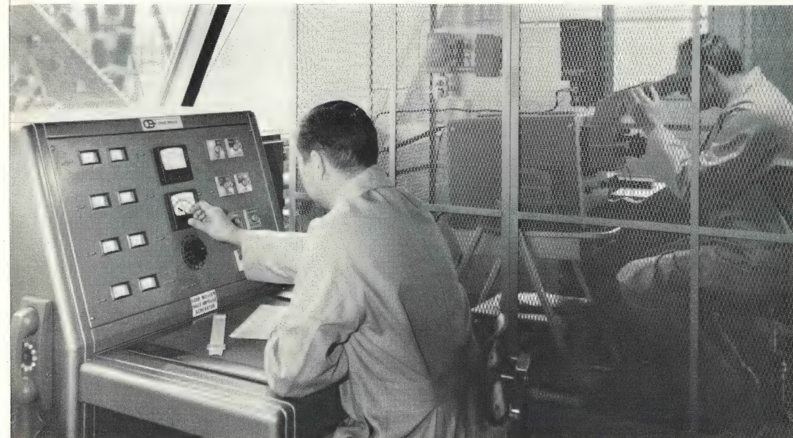
Transmission line prototypes are extensively investigated on O-B's new 4,000-kv outdoor weatherproof impulse generator. Accurate test readings are a prime requirement in this class of work. High energy impulse generators are capable of supplying large ground currents following a flashover. This will produce ground voltages which can cause oscillograph interference if a shielded screen room is not used.
