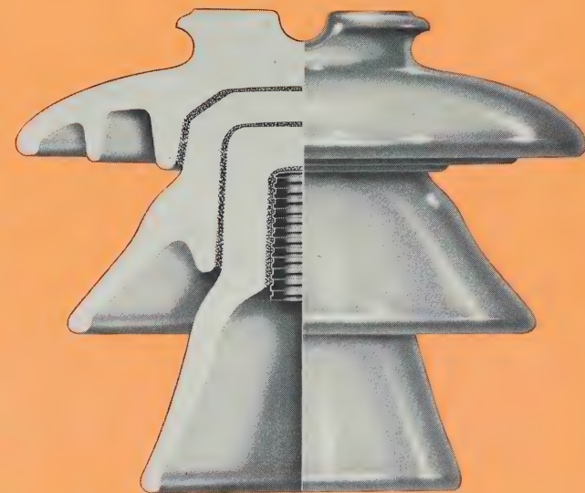
Section view of O-B multipart insulator illustrates the stacked assembly of three concentric porcelain shells which produces operating superiorities.
