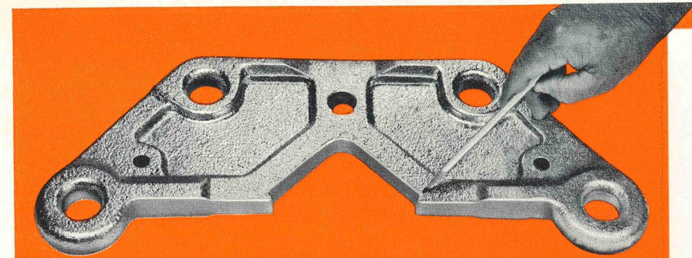
A Small, accurate details, such as positioning points for hot-line tools, are faithfully reproduced by the casting process. Other common shaping methods cannot form a part with such fidelity.
