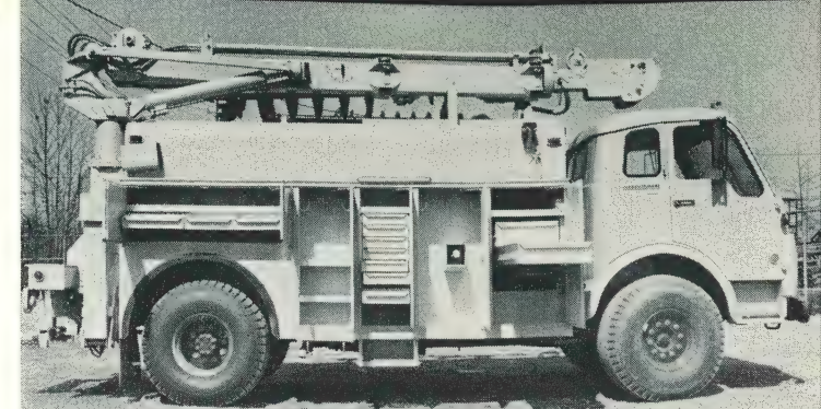
Shifting compartments for rubber goods, winch and various hardware forward helped redistribute weight to front axle.
