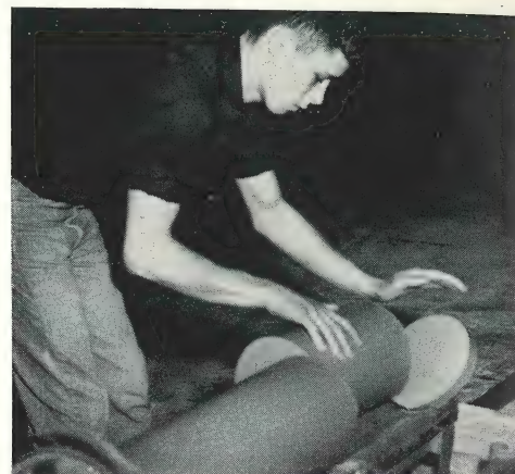
Clay blanks are extruded for future trimming into station posts.
