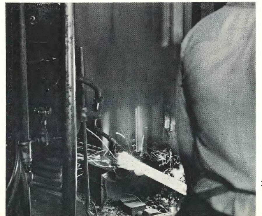
6 — Molten non-ferrous metals all pass this station where exact pouring temperature is confirmed by pyrometer measurement.
