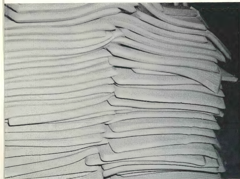
Clay filter cakes weigh approximately 38 pounds. Each cake is a dense mass of clay, shaped into a giant molded square.
