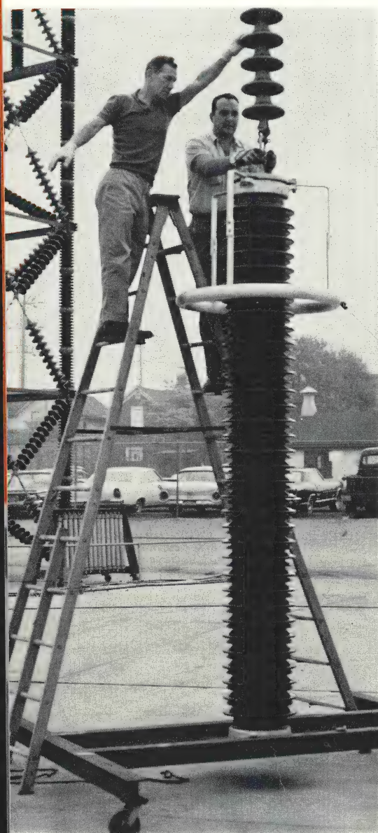
Figure 1 — Dynagap 5 arrester is suspended on insulator string and elevated to testing position in O-B's High Voltage Laboratory.
