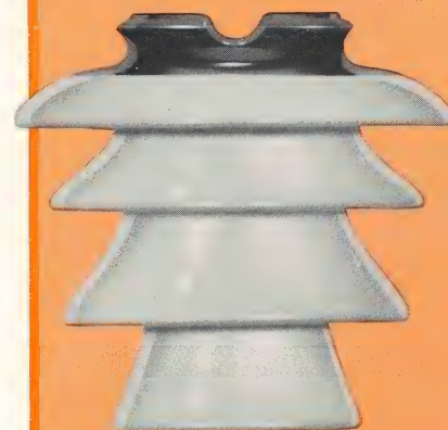
Tietop multipart pintype insulator for severe duty on 69-kV circuits. Extra leakage is obtained by the addition of a fourth skirt.
