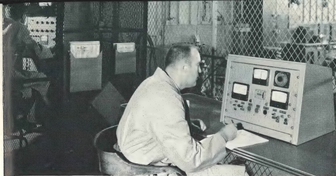
For quality control, inspection, and other long product testing runs, a special impulse generator is assigned to this work to relieve larger equipment used primarily in research. From time to time precise data is required from this department, especially in analysis of factory production, and for this purpose the oscilloscope is carefully shielded in its clean room, shown in the background.
