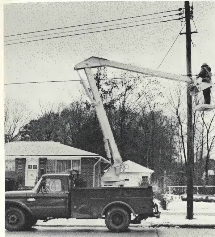
Three different models in two bucket heights — 27 or 31 feet — offer you new flexibility for light-duty applications in Holan's new Bronco 87 series. Its single bucket furnishes a manload lifting capacity of 300 pounds.
