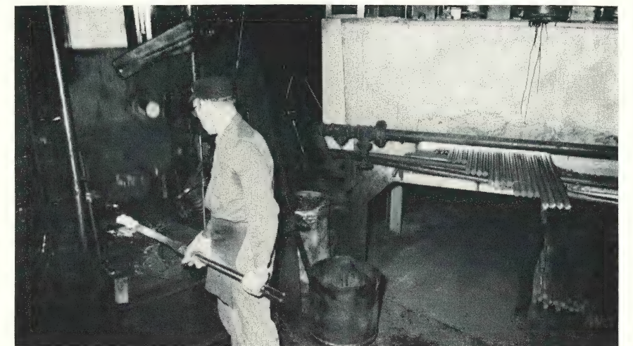
8 — Drop forging a steel suspension insulator pin. Heating ovens maintain correct temperature so that the metal stock receives a thorough "soaking" at a specific heat before and immediately preceding the forging operation.
