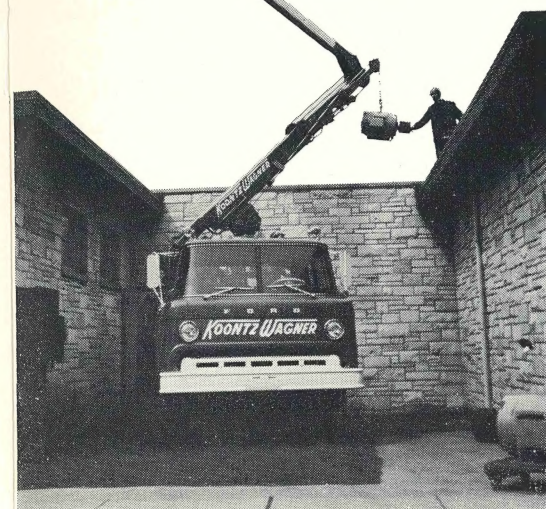
For heavy material handling, select a lower-arm "stinger" boom with hydraulic winch that provides lift capability up to 6,000 pounds for your Bronco 89.
