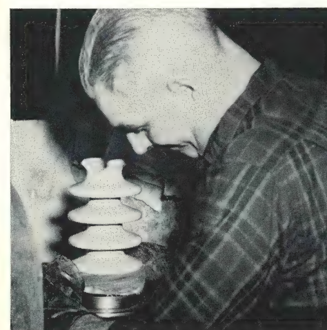
Line post receiving final cleaning.
