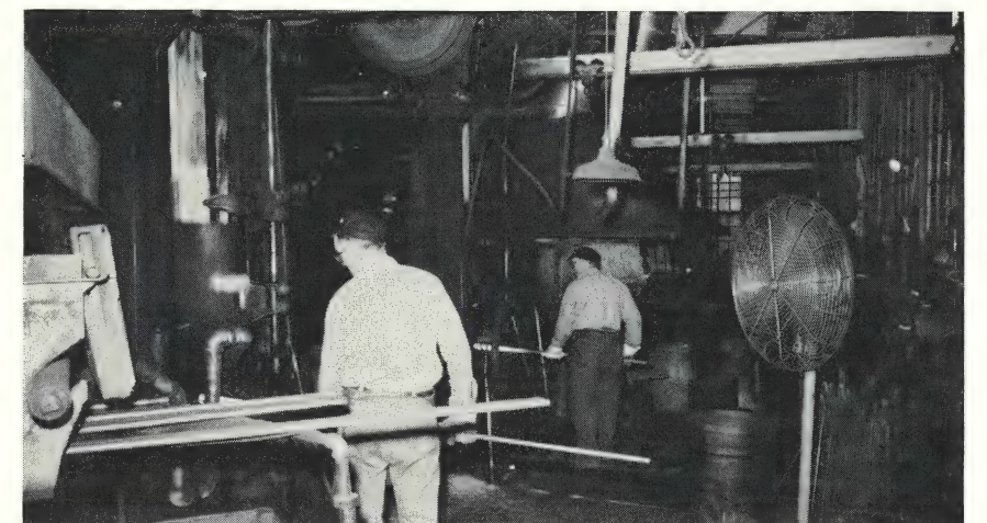
9 — Part of the line of drop forges in the O-B shop. As one progresses down the line he will see a series of forges of graduated capacity, permitting lighter, faster machines to be employed for smaller pieces.
