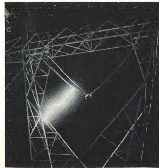
Outdoors, a surge produces a gap flashover to the side of a full-scale tower erected in the test yard. Testing the full-scale final design proves the validity of your design criteria and gives you detailed performance information before construction.
