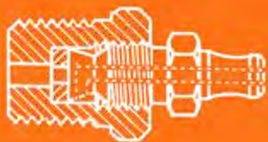
A simpler version of a sampling device is Number 5710. Slip connection for a sampling tube remains exposed while not in use. A light turn on the hex nut opens and closes the sealing disc.
