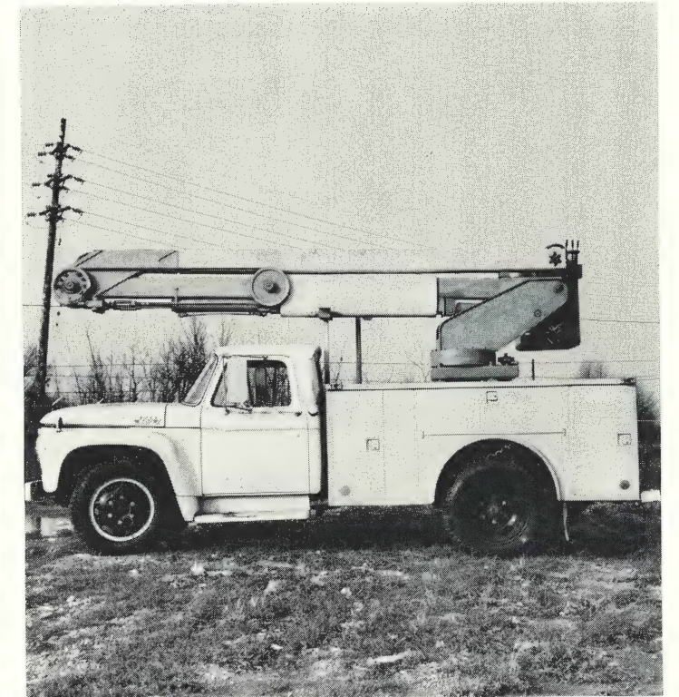
Holan's Bronco 89 series offers two new bucket heights to round out the Holan product line. Available in 36- and 41-foot bucket heights, this new material-handling unit offers an optional fiberglass-reinforced plastic insert in the lower arm.
