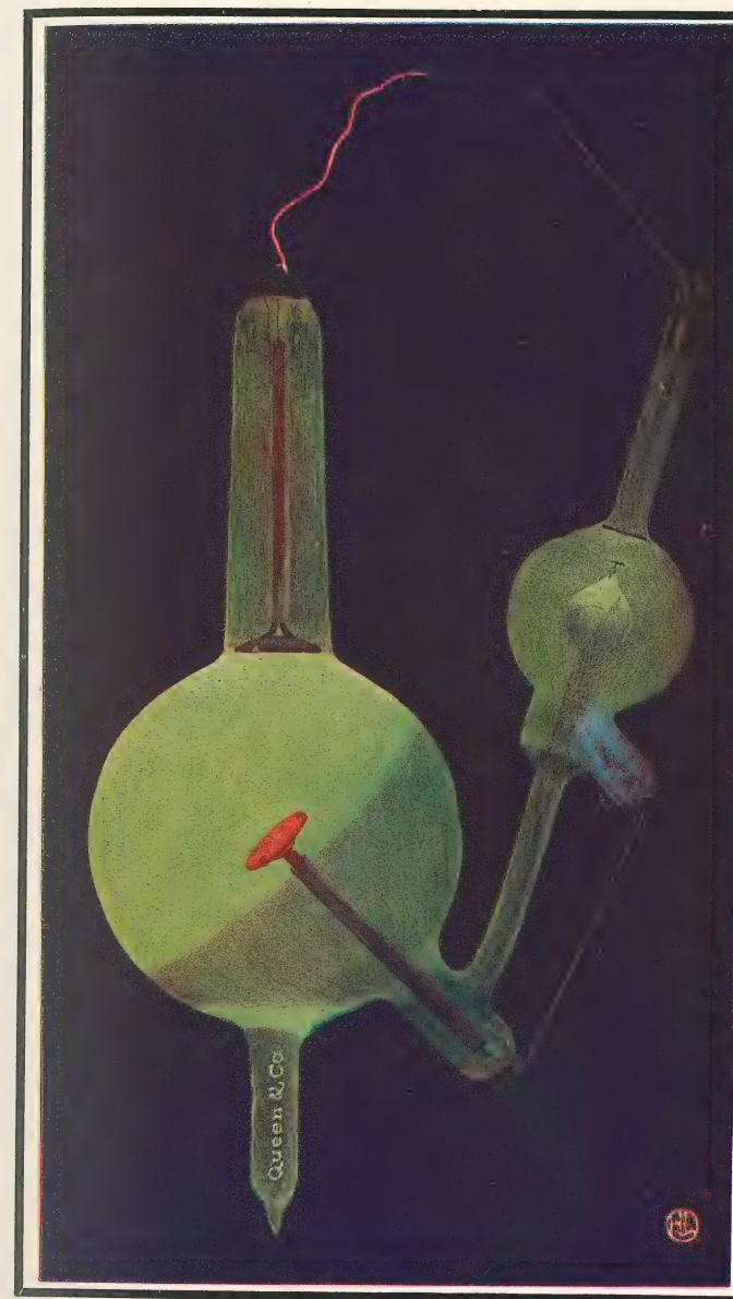
SELF-REGULATING X-RAY TUBE. OPERATING PROPERLY.
