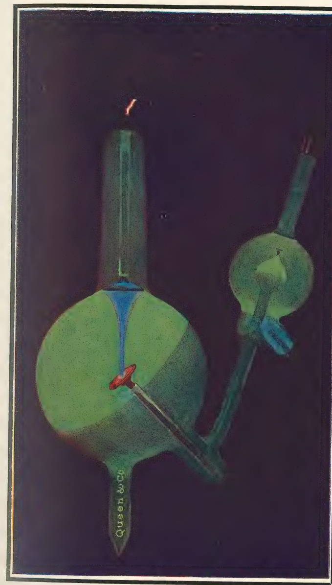
SELF-REGULATING X-RAY TUBE. LOW VACUUM. (FIG. 96.)
