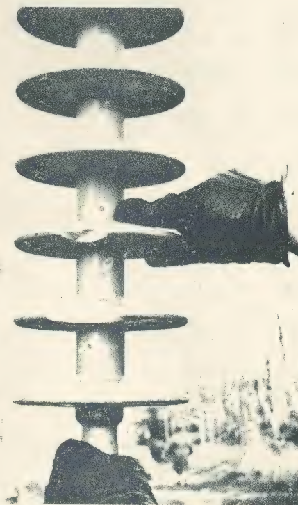
Fig. 4. Polymer Insulator after being subjected to direct hit from a .45 calibre service pistol.
