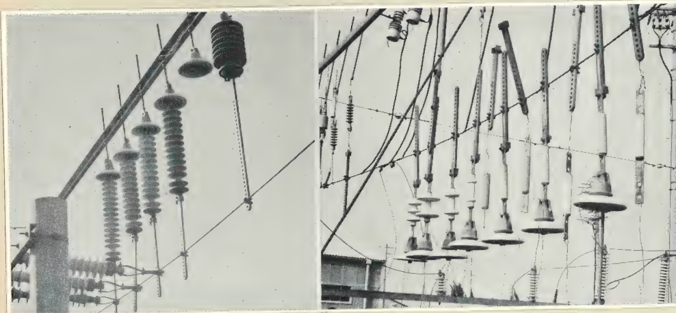
(c) Test Pieces of Various Resins (applied voltage 6kv)
