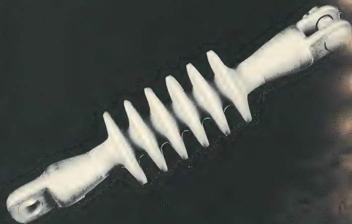
Fig. 1. The new lightweight 15-kv GEPOL suspension insulator features very high impact strength polymer body with long leakage distance and a fiber-glass rod for mechanical support.
