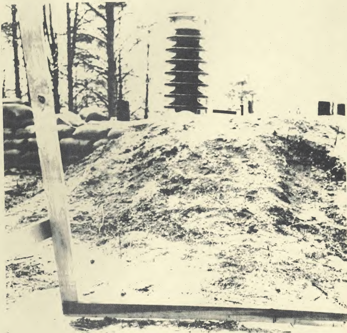
Lapp Strut - 45 cal. pistol - broke bottom insulator (1 shot).
