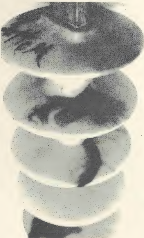
7. GEPOL Insulator Tracked on Field Trial
