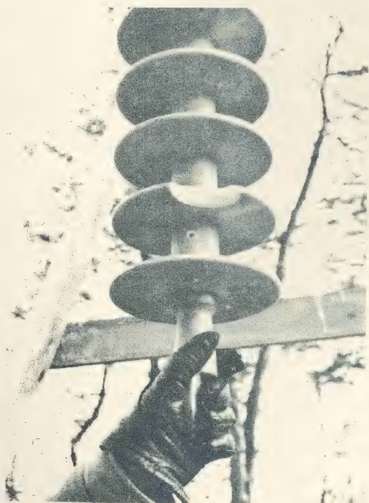
Fig. 3. Polymer Insulator after receiving direct hits from .22 calibre long rifle fire at 50 feet.
