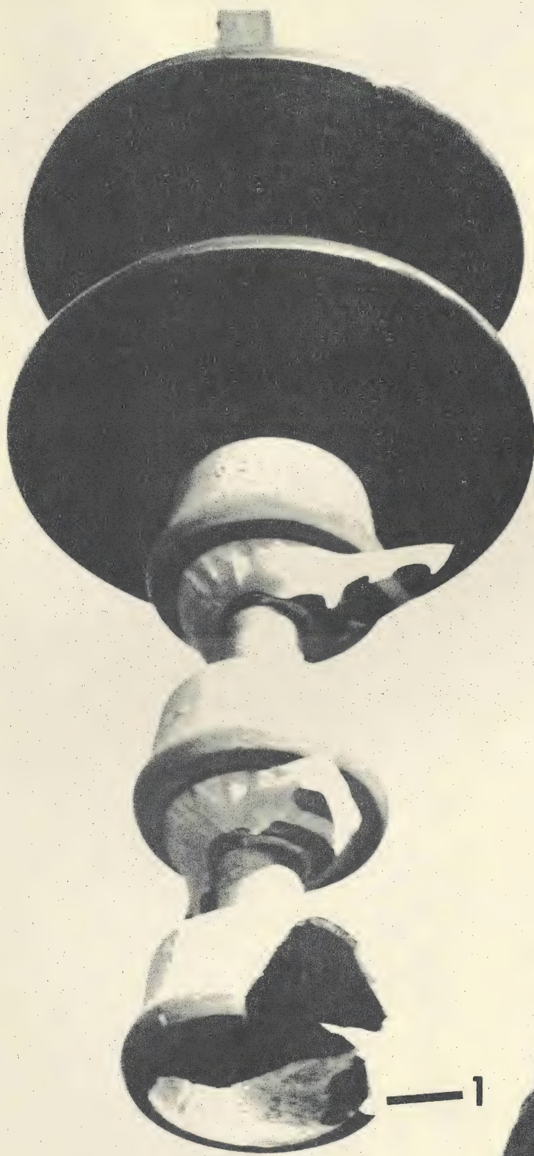
Locke Unispar - M-1 rifle - 3rd direct hit into hole in cap split head of insulator and dropped the lower half of the unit (1 shot).
