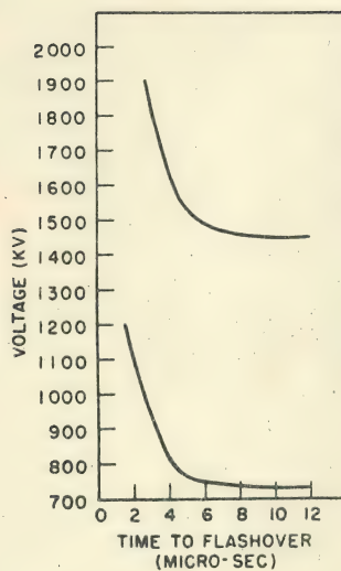
Fig. 8. Volt time curves for one and two polymer insulators, positive polarity.
