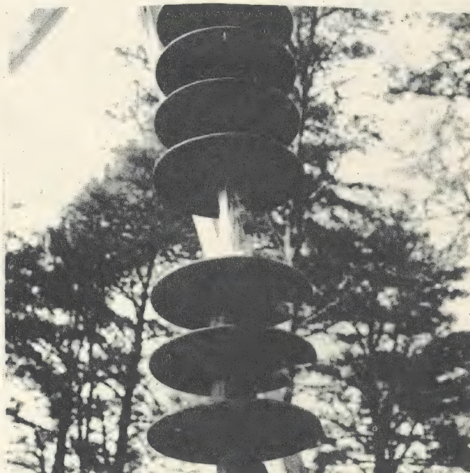
FIG. 4 --- .30/06 CALIBRE RIFLE DAMAGE
