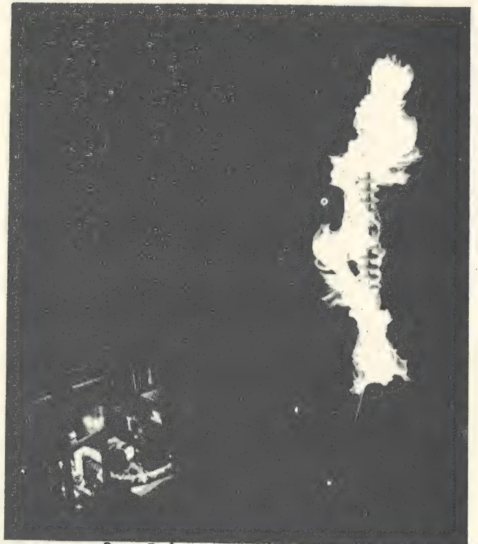
8. Laboratory Flashover Test - GEPOL Insulator
