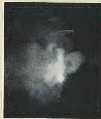
(a) Power arc test 4,000 A x 30 cycles
