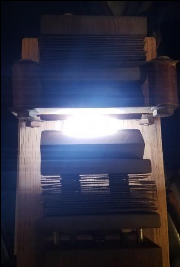
Iron Spark Condenser Discharge Lamp (Thomas Burton Kinraide, Patent 1904) (Replica built by author.)
