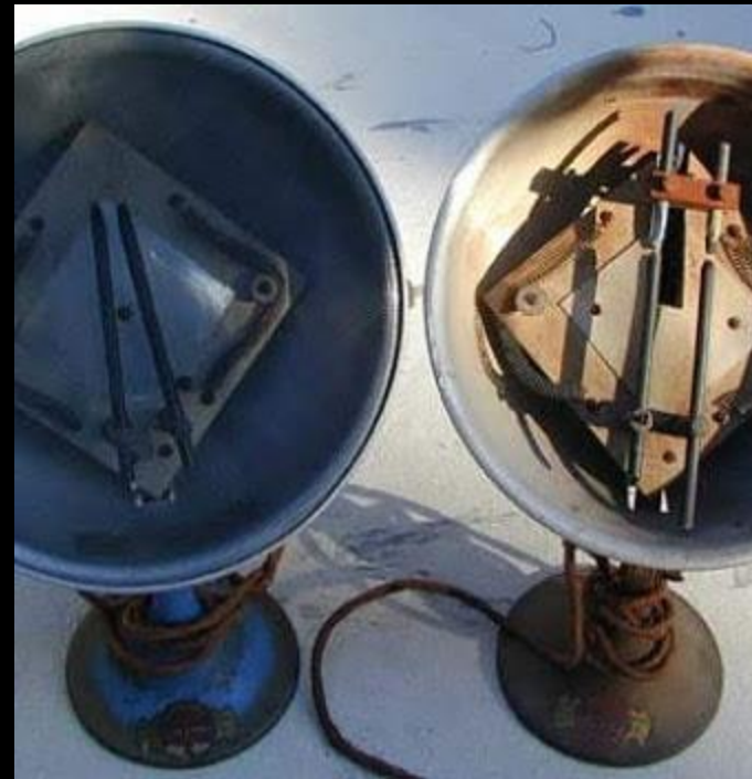
Carbon Arc Lamps (First demonstrated by Sir Humphrey Davy in 1807, perfected for lighting in the 1870s)
