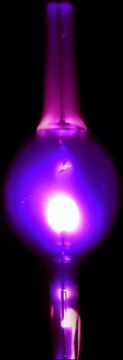
Swett & Lewis X-Ray Tube with low vacuum (1897)
