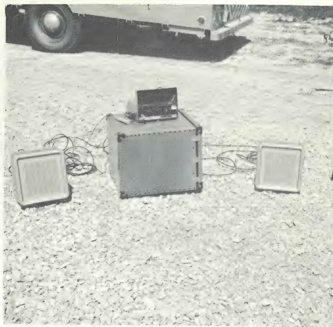
Figure IV-12. Portable Amplifier and Speakers Used by Crews for Ground to Tower Communications.
