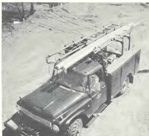
Figure IV-18. View of Pick-Up Truck Used to Tow Trailers and Transport Larger Length Sticks and Ladders.
