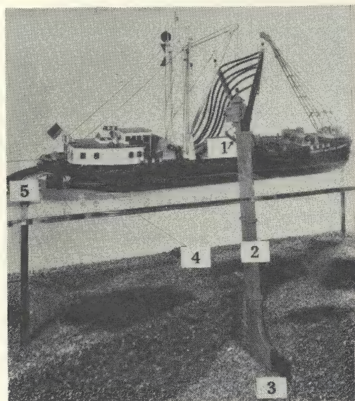
HYDRO-JETTER UNIT: 1-water-pressure hose; 2-injector; 3-plastic conduit to be embedded in river bottom; 4-winch line; 5-free-running conduit coils
