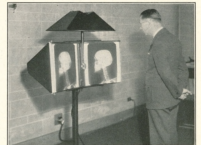
Arrangement of Stanford Pedestal Stereoscope for use as view box.
