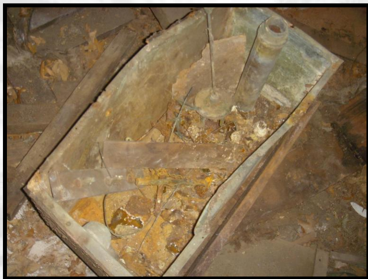
Remains of the copper-lined oak box that contained the oldest oil-filled high frequency coil of Kinraide's design. Found with Stephen Hadley in 2007. This coil was documented in Frederick Finch Strong's book High-Frequency Currents (1908).
