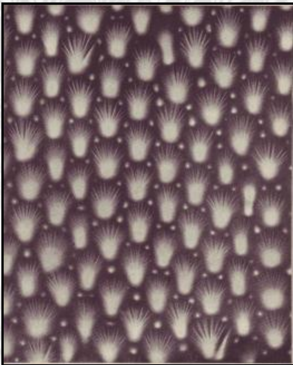
PLATE VII. NEGATIVE ENDS OF ELECTRIC ENTITIES. A discharge from a metallic roller iii its passage over the film side of a photographic plate placed upon the uncoated, positive surface of a charged condenser. This plate is a companion to Plate VI.
