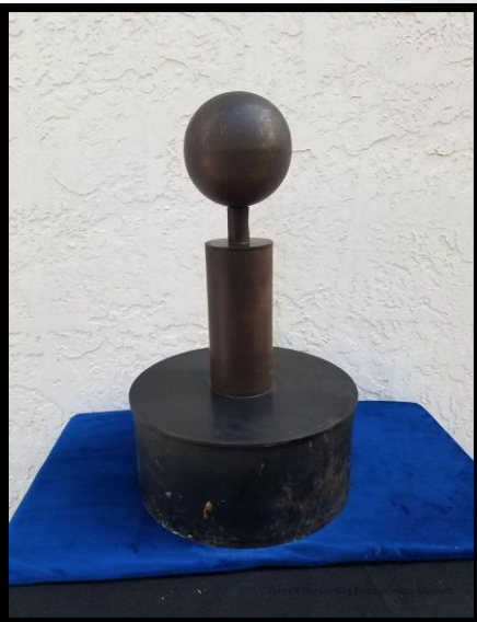
Original and early prototype Kinraide Coils from Ravenscroft to make electrographs
