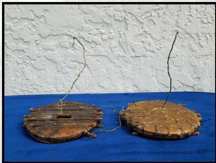
Original and early prototype Kinraide Coils from Ravenscroft to make electrographs
