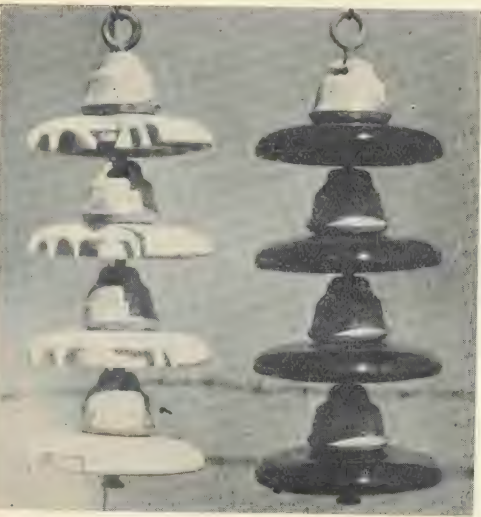
Fig. 10. Comparison of impact resistance of insulators with glazes in tension (left) and in compression (right)
