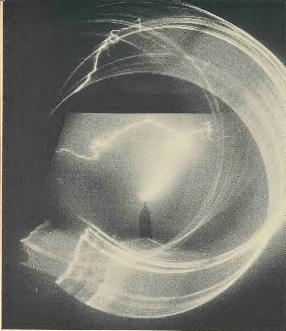
Long-continuing upward leader stroke showing upward branching. Part of left branch is cut off by window at beginning of rotating image. Period of streamer build-up is clearly shown at beginning of discharge. After this period is over, discharge becomes almost steady direct-current arc with heavy current-peak at end. Total time of discharge is 0.616 second. Charge in coulombs is 99, much above average in New York.
