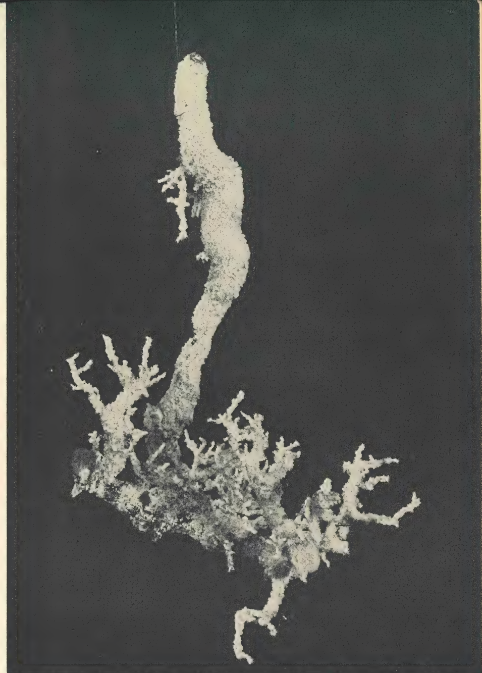
Fulgurite made in High-Voltage Laboratory at Pittsfield by F. W. Peek, resulting from flow of a few amperes at high voltage through sand. Current was maintained until sand melted to form fulgurite. Low-current discharges persisting for about one second cause formation of similar fulgurites as the result of natural lightning discharges.
