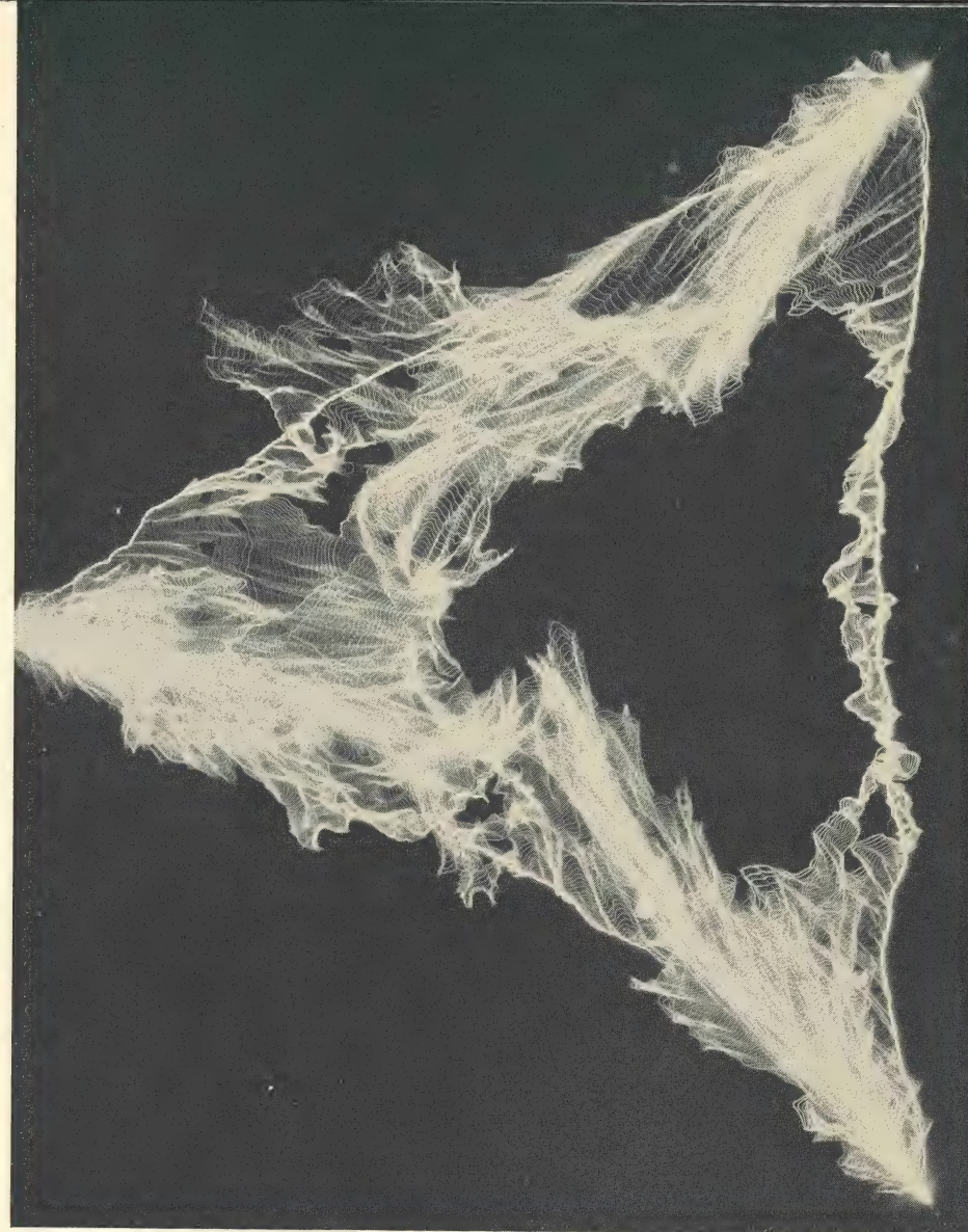
Time exposure taken from above of a 1,000,000-volt three-phase 60-cycle arc between points separated 108 inches. Note changing path as discharge rises. Fine lines result from alternating potential changing polarity 120 times per second.
