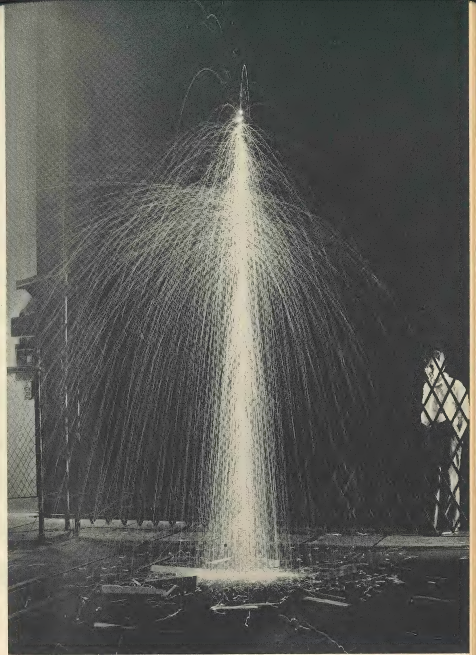
What happened to a No. 25 nichrome wire when current from a 5,000,000-volt generator was passed through it. Current must be adjusted carefully to give this effect since too much current eliminates wire without shower of sparks seen here.
