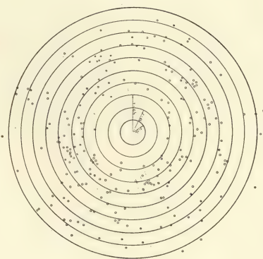
Record of strikes to plane surface with one-half-inch needle-point at center of circles. Cloud (represented by sphere) is directly over needle. There are no strikes within an area whose radius is equal to four times height of needle.
